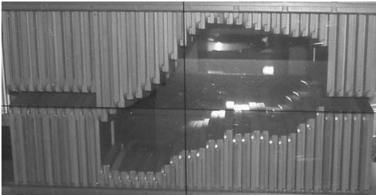
Figure 9.1 The leaf pairs of a multileaf collimator (MLC).
