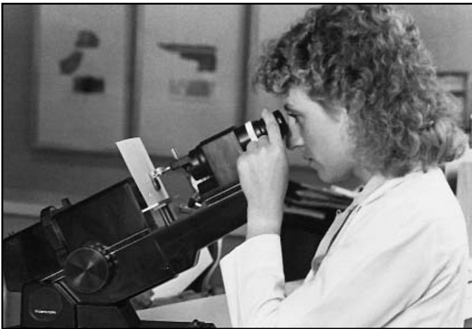
Figure 3-2. A white piece of paper provides an excellent background for eyepiece adjustment. (Photo by Mark Arrigoni.) (Reprinted from Her-rin MP. Ophthalmic Examination and Basic Skills . Thorofare, NJ: SLACK Incorporated; 1990.)
