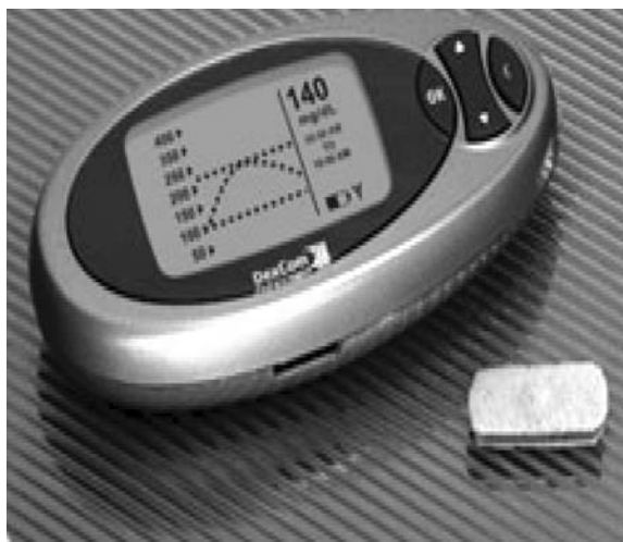
FIGURE 5 Electrochemical ISF glucose sensor designed for long-term implantation within the subcutaneous tissue. ISF glucose data is transmitted wirelessly to the patient-worn display (mg/dL versus time) ( www.DexCom.com ).
