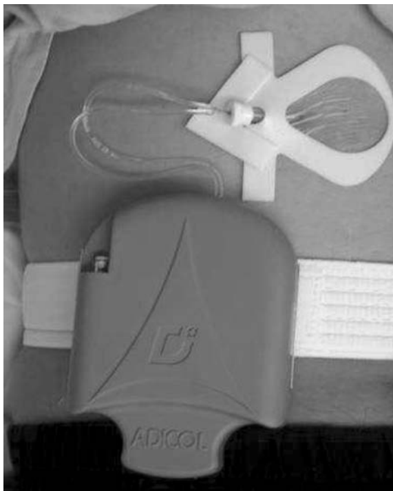
FIGURE 4 Dialysis catheter-type CGM system. Flexible small-pore catheter is connected to an external flow through electrochemical glucose sensor, following insertion into the subcutaneous loose connective tissue ( www.ADICOL.com ).
