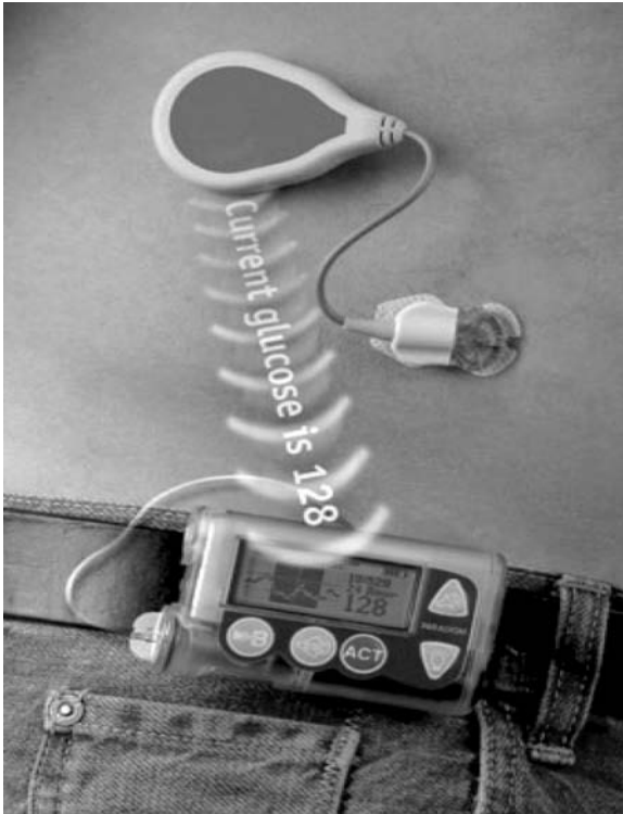
FIGURE 7 Medtronic Diabetes (Guardian REAL-Time) CGM System. Distal tip of needle-type glucose sensor is implanted into the subcutaneous tissue of the abdomen. Glucose data is sent wirelessly from telemetry module to insulin pump. Glucose data displayed on y-axis and time of day on x-axis. CGMS is open-loop system, requiring patient initiated SMBG for change in insulin dose ( www.medtronicdiabetes.com ).
