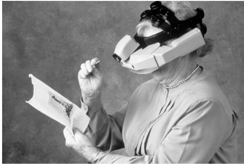
Fig. 54.3. The Low Vision Enhancement System (LVES), developed at the Lions Vision Center (Johns Hopkins University), with support from NASA and the Department of Veterans Affairs, is a characteristic example of optoelectronic vision enhancement systems. This system features binocular orientation cameras, a centrally placed 1.5–10× zoom camera with automatic focus, and a binocular projection path with built-in refractive correction and alignment for the wearer.
