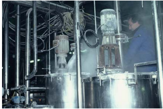
Plate 8: Filling up vats with polyvinylpyrrolidone powder by an operator in a brewery.
