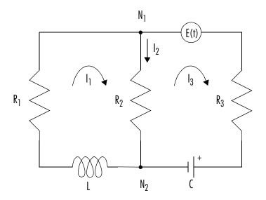
Let Rj and Ij, j = 1, 2, 3 be resistances (measured in ohms) and currents (amps), respectively; L be inductance (henrys), and C be capacitance (farads); E(t) be the electromotive force, and Q(t) be the charge
