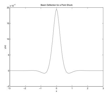
shows that the impact of a blow on a beam is highly localized; the greatest deflection occurs at the point of impact and falls off sharply from there. This is the behavior we expect from experience.
