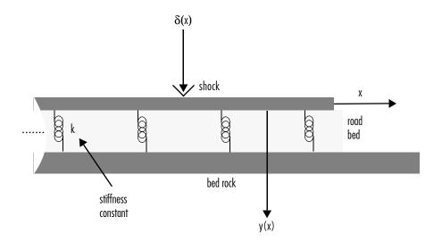
The shock could be induced by a pneumatic hammer blow (or a swing from the mighty John Henry!).
