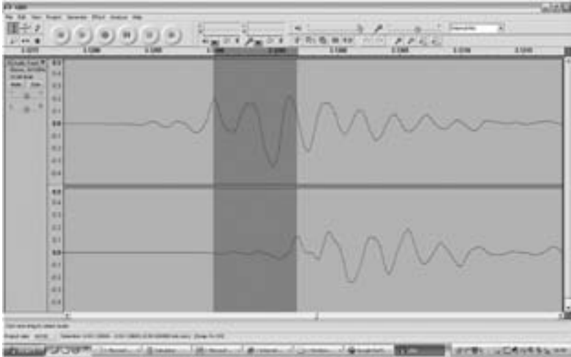
FIGURE 19.1 Typical Result for Speed of Sound Measurement Using Audacity
