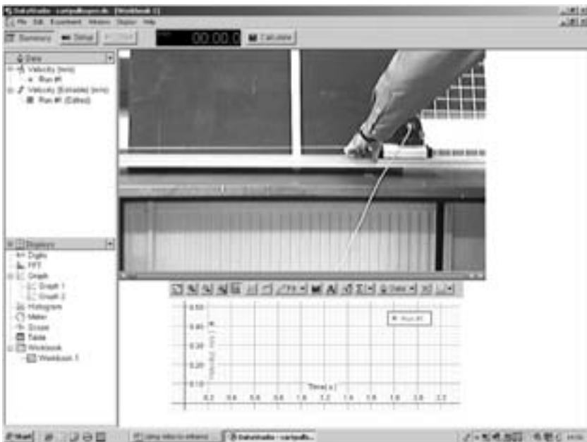
FIGURE 18.5 Showing Video Data for an Experiment with Data Logged with a Motion Sensor
