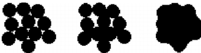
FIG. 18. The evolution of a collection of circular particles (left to right) under the sintering algorithm described in the text.
