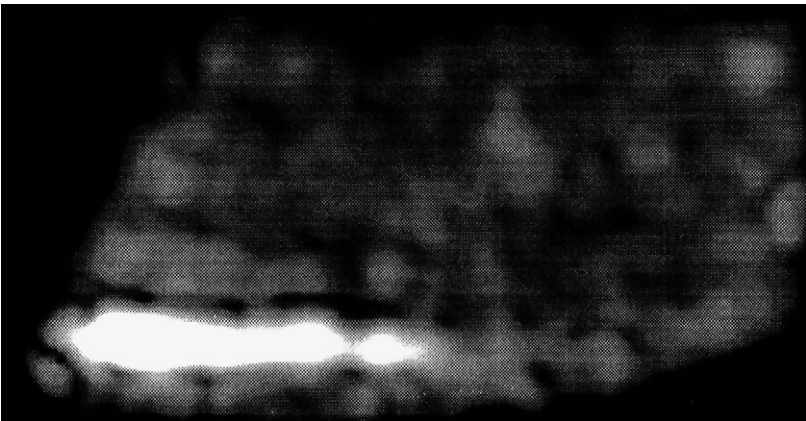
FIG. 13. Slow wave image of a 1- × 2-in., 1.1-mm-thick Berea sandstone sample of 400 mD average permeability at 210 kHz. Reprinted with permission from P. B. Nagy, B. P. Bonner, and L. Adler, Geophys. Res. Lett. 22, 1053–1056 (1995).
