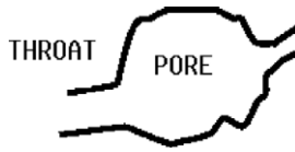
FIG. 2. Schematic picture defining a throat and pore in the pore space of a porous material.
