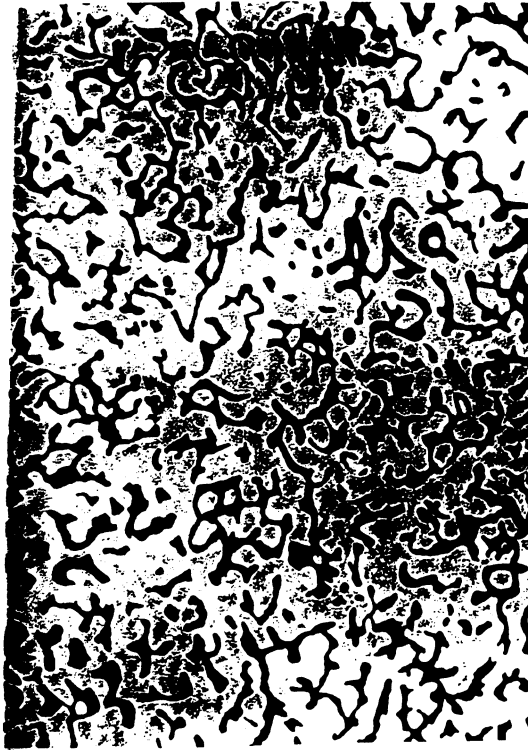
FIG. 4. Transmission electron micrograph (TEM) of a thin section of Vycor glass. Reprinted with permission from P. Levitz, G. Ehret, S. K. Sinha, and J. M. Drake, J. Chem. Phys. 95 , 6151. Copyright 1991, American Institute of Physics.
