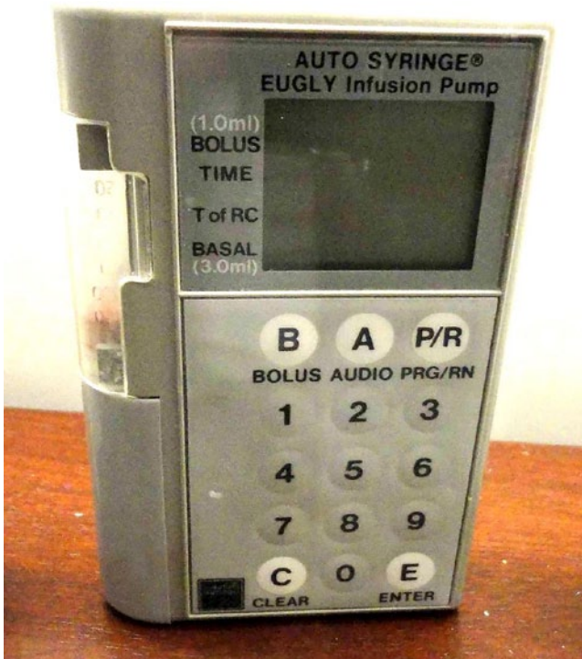
FIGURE 6.6 Early insulin pump AutoSyringe. © Bill Van Antwerp.
