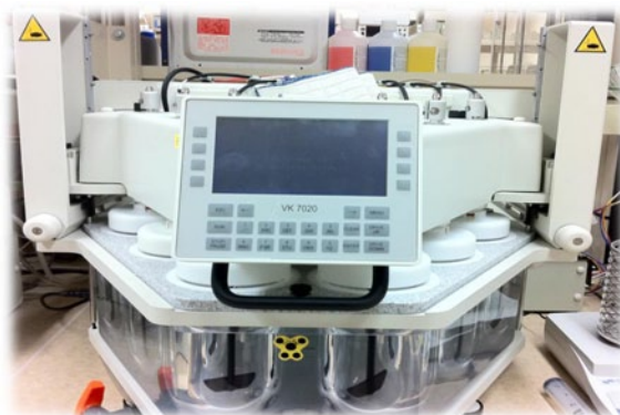
FIGURE 12.2 Apparatus 1 and 2 dissolution test.
