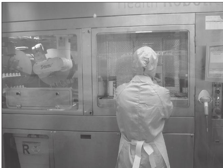
Figure 6.5 Automated filling equipment system, Imperial College Healthcare NHS Trust.
