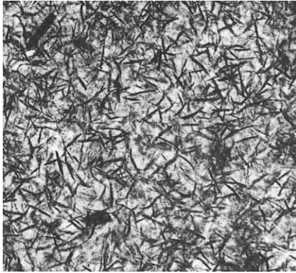
Figure D.1.4. Clear oxide layer formed on 3003 by immersion in boiling distilled water ( 50\,000\times ) [9].
