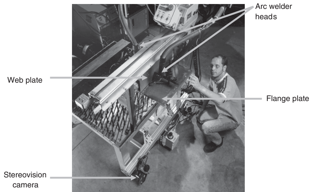
6.8 Overview of experimental setup for welding the T-section plate.
