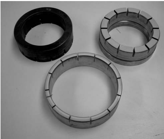
FIGURE 3.8 Various condition rings used in lapping process. (From www.engis.com .)
