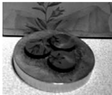
FIGURE 4.41 Example finished by #20000 wheel.
