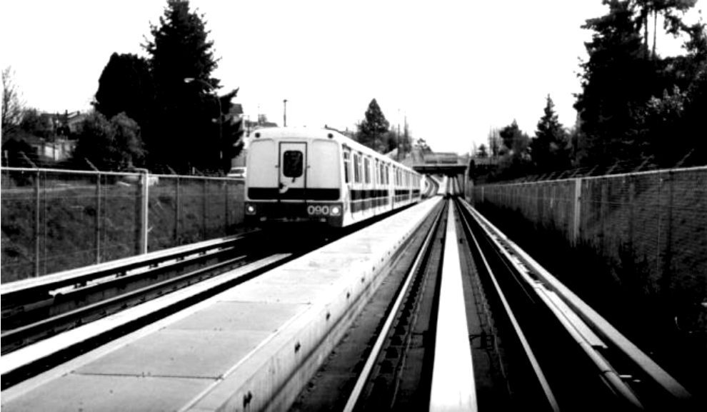
Figure 1.15 The BC transit system in Vancouver: with linear motion induction motor propulsion (source: UTDC)
