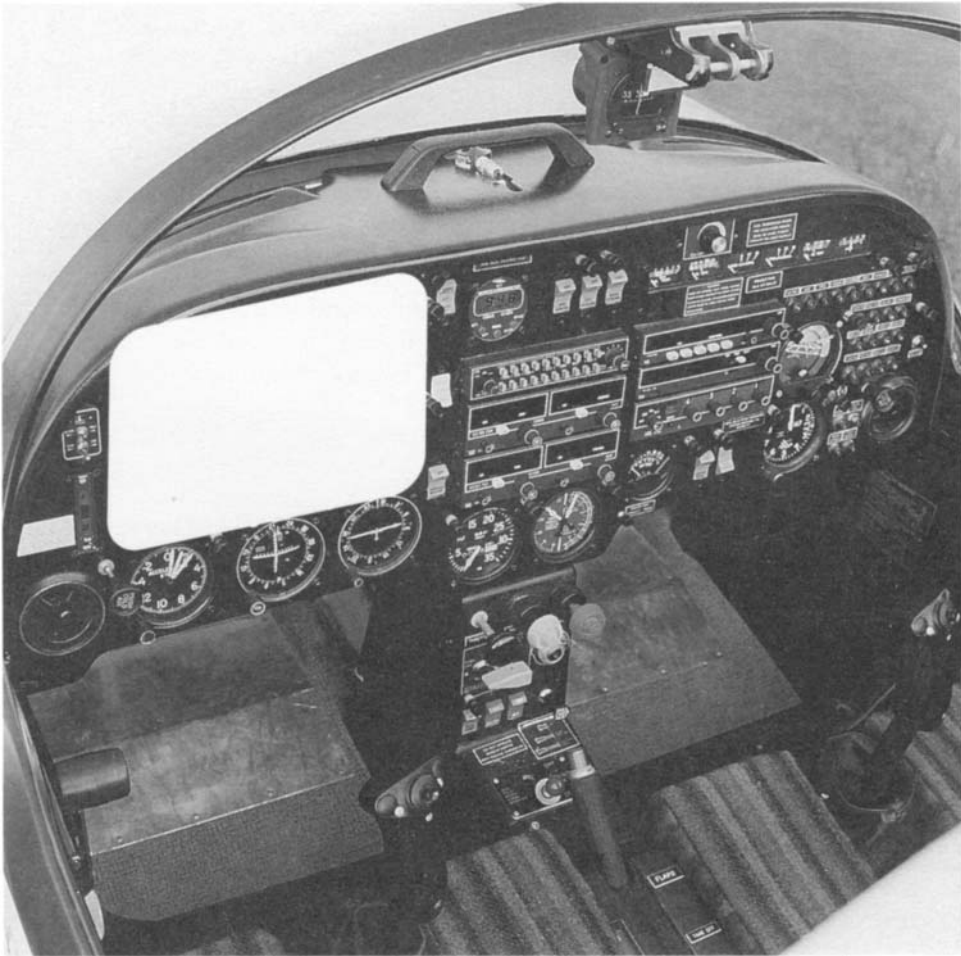
Figure 13.6 Cockpit layout – showing space for flight instruments (courtesy Slingsby Aviation Ltd, UK)
