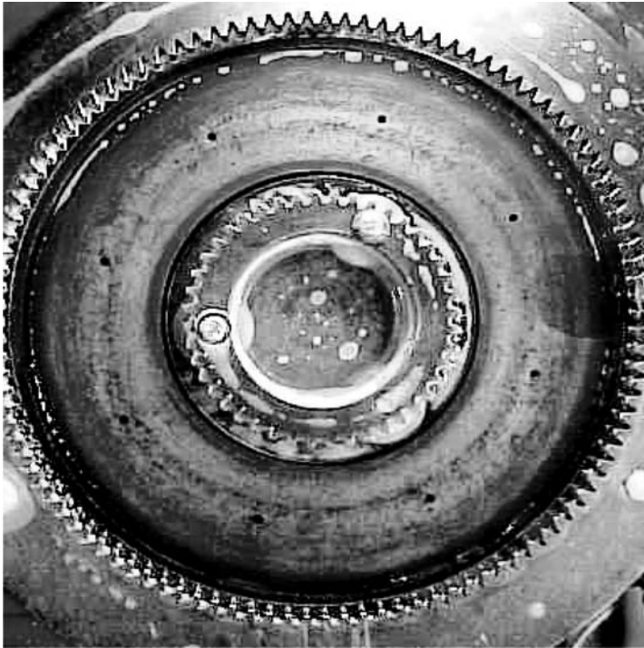
FIGURE 12.12 Radial wear gradient of the diamond wheel.
