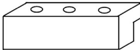
Figure 12.7 Retaining feet blocks for splits
