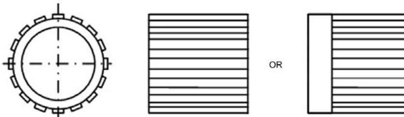
Figure 13.20 Typical serrated form on part to prevent part rotation
