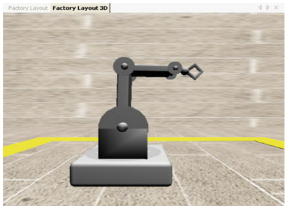
Fig. 1.29 Virtual model of a revolute robot
