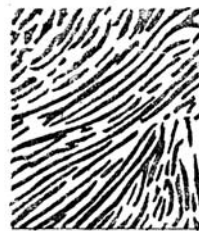
Fig. 8.2 Micro structure of pearlitic eutectoid steel
