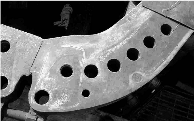
Figure 17-20. Picture of the flange face of the casing. Note the unevenness caused by past hot air leaks. The deep narrow groove is caused by previous attempts to stop the leak by crushing a wire between the two flanges.
