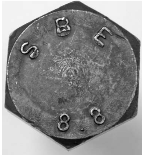
PHOTO 12.1 A general purpose metric fastener can be identified by the number (8.8) showing the strength level.
