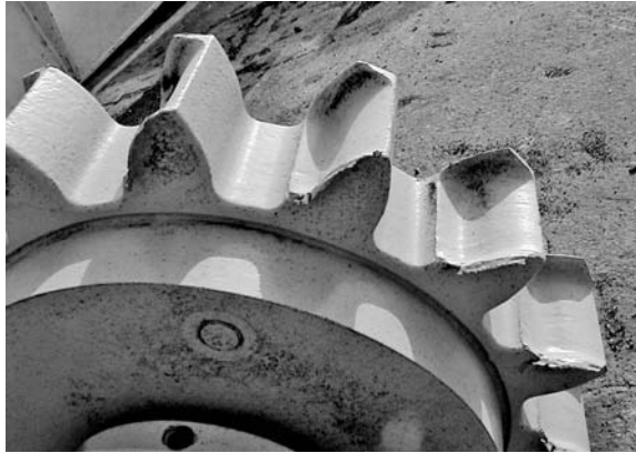
PHOTO 8.3 Abrasive wear of a large engineered chain sprocket.
