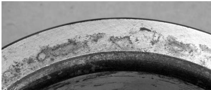
PHOTO 10.7 The black marks on the side of this inner ring are proof that water has been present.
