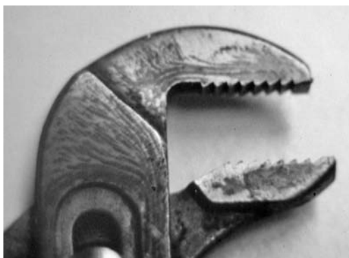
PHOTO 7.1 Uniform corrosion of a forged piece, showing anode and cathode areas.
