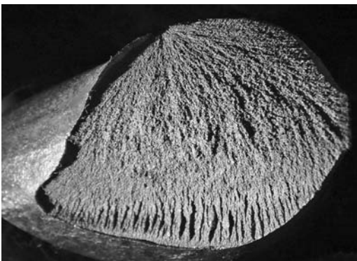
PHOTO 4.11 Easy to identify failure origin because the low light angle accentuated the Chevron marks.
