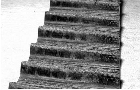
PHOTO 9.6 The underlying construction fabric on the right side of these synchronous belt teeth is showing, and the uneven wear is obvious evidence of misalignment.
