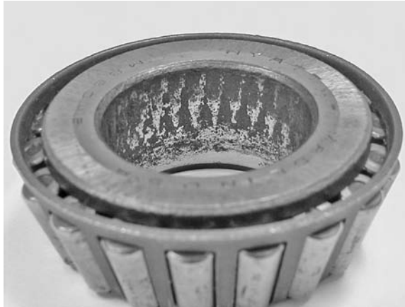
PHOTO 10.13 Another very loose fit complicated by the grinding pattern.
