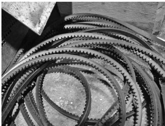
PHOTO 9.5 This is a pile of belts that has just been removed from a large fan. The elastomer on the sheave contact surfaces is shiny and polished, proof that the belts have been slipping.
