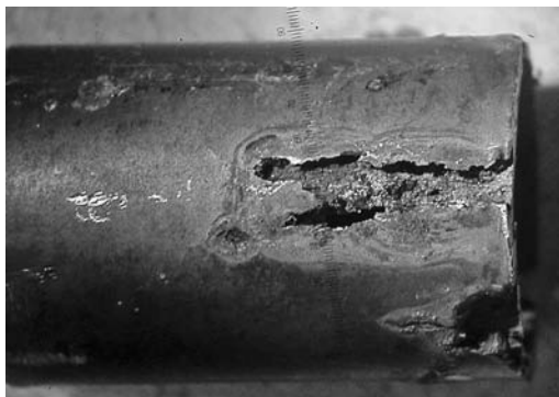
PHOTO 7.14 Crevice corrosion damage on a 304 stainless tube that was up against another piece of type 304 stainless.
