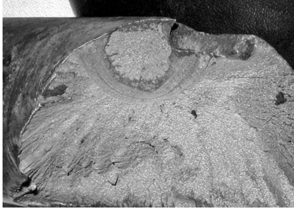
PHOTO 6.14 An oven chain drive shaft with an unusual surface appearance.
