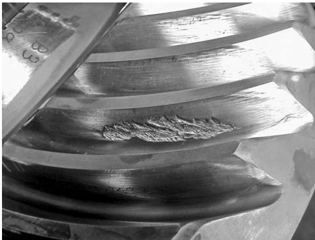
PHOTO 11.18 Spalling of an intermediate spiral bevel pinion — the result of a manufacturing problem.
