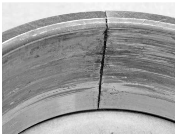
PHOTO 10.2 This shows the shaft fit from a through-hardened bearing. The crack extends to the rolling surface and a catastrophic failure is not far away.
