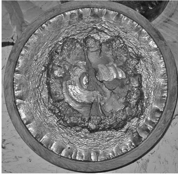
PHOTO 6.13 This low cycle torsional fatigue failure saw more stress cycles than the previous shaft.
