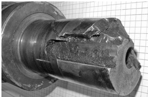
PHOTO 6.4 The constant hammering from the loose coupling fit and the torsional fatigue forces both wore the side of the keyway and caused a crack that started at the keyway root.
