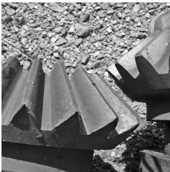
PHOTO 11.11 A through-hardened steel mill gear with heavily worn teeth that show rolling damage.
