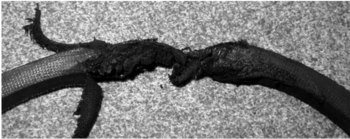
PHOTO 9.9 Spin burn damage on an A section belt. In this case, the machine jammed and the belt tension was so loose that the drive sheave slipped and heated the belt literally until it charred. This damage is common when a machine jams but it can also happen from lack of tensioning. During operation, a belt constantly stretches and, on a machine such as a fan, when the tension ratio goes over about 16 (5% slip), the chance of this happening increases rapidly.
