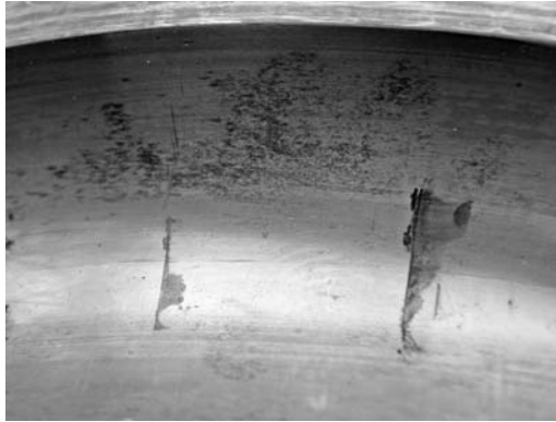
PHOTO 10.6 The two black lines are water spots (corrosion damage) on a ball path.
