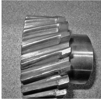
PHOTO 11.8 Wear of a through-hardened pinion with less than 50% of the tooth remaining.
