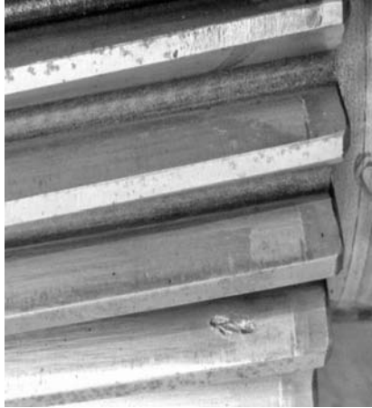
PHOTO 11.15 Micropitting from misalignment plus a pit, in this case hardened gear.
