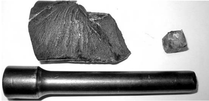
PHOTO 4.2 Torsional overload failures of a through hardened truck axle and an inexpensive socket wrench extension. Note the difference in appearance.
