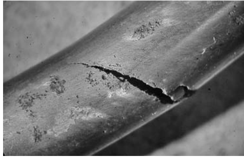
PHOTO 7.22 The SCC cracks started from a series of small pits.
