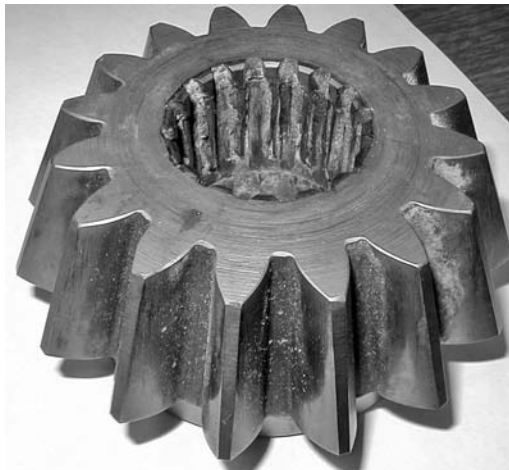
PHOTO 11.2 A bevel gear — essentially a spur gear for right-angle drives.
