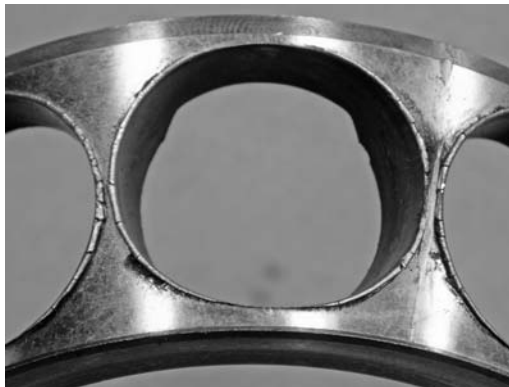
PHOTO 10.38 A bronze cage showing plastic deformation resulting from torsional vibration and marginal lubrication.
