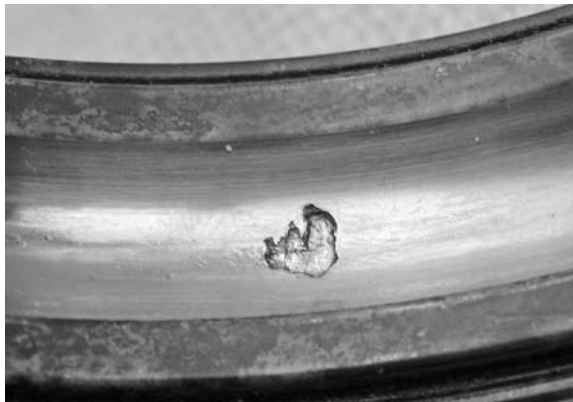
PHOTO 10.25 Another Hertzian fatigue spall.
