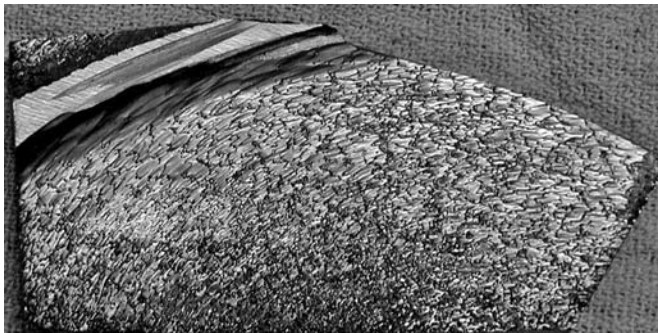
PHOTO 7.11 Erosion corrosion of a pump impeller.
