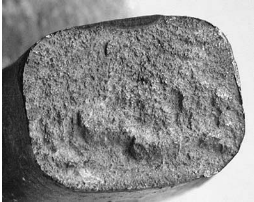
PHOTO 2.3 A brittle fracture that originated at a surface defect.
