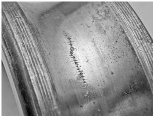
PHOTO 10.36 This pump bearing was rotating when the welding arc left this tell-tale track.
