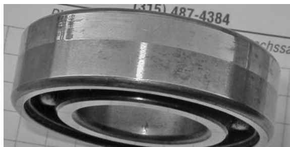
PHOTO 10.8 The design called for only ½ of this bearing to be supported — and the fit was very loose.
