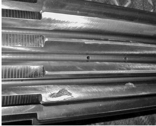
PHOTO 11.21 The large spalls on this pinion lead one to suspect a metallurgical problem.
