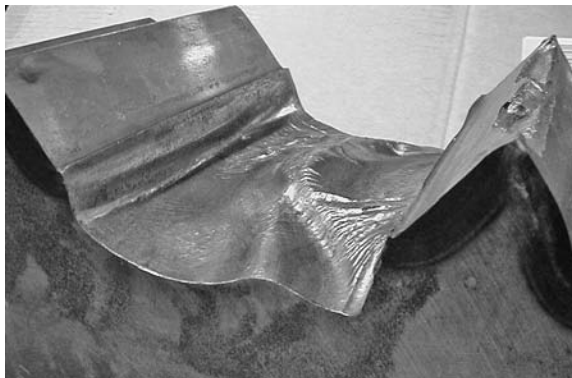
PHOTO 11.20 The river marks in the failure face show this cracking progressed from left to right.
