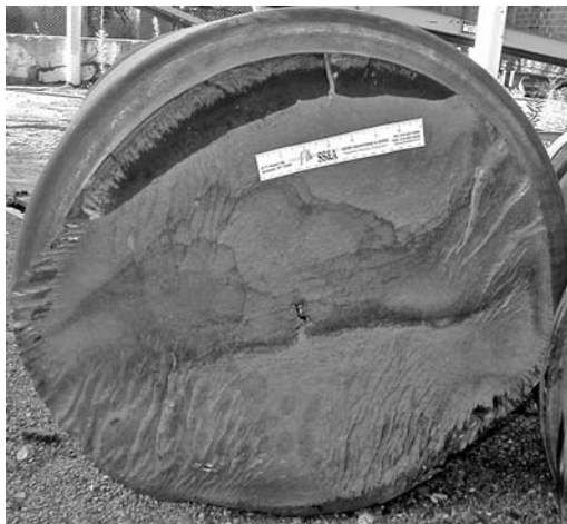
PHOTO 6.11 A roll from a steel mill. The blackened area is an older oxidized crack surface. The IZ is the lower third of the roll.
