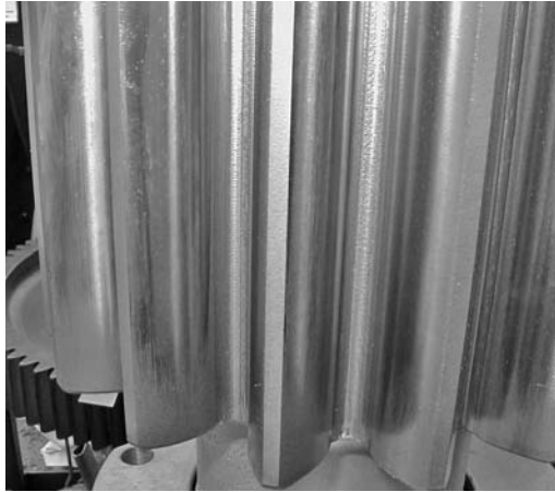
PHOTO 11.6 The contact pattern testifies to the misalignment of this case-hardened pinion.
