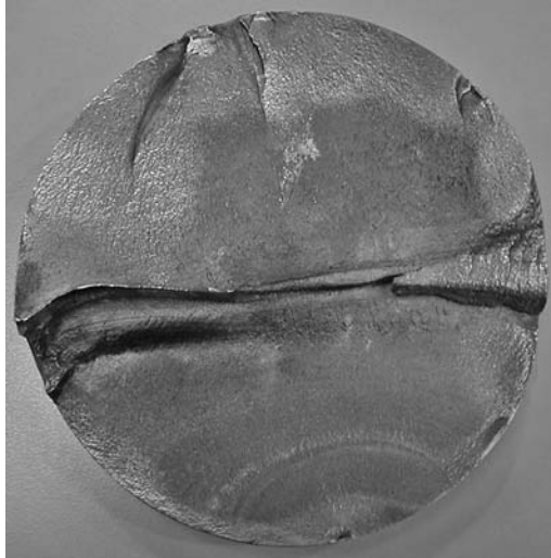
PHOTO 2.1 Fatigue failure of an agitator shaft.
