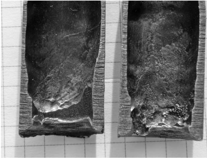
PHOTO 7.10 Erosion corrosion of two heat exchanger tubes.
