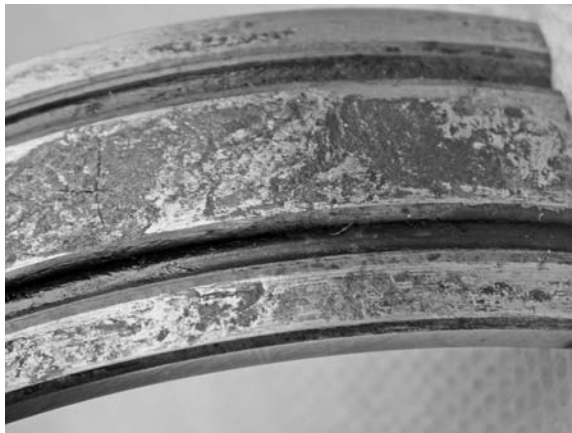
PHOTO 10.14 A heavily fretted surface with a visible crack.
