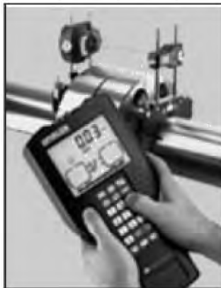
Figure 6.35 Laser alignment system comprising of laser head, reflector and analyzer (Prueftechnik – Optalign Plus system)
