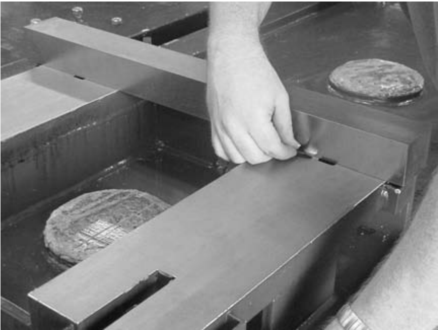
Figure 3-37. Flatness and coplanar check.
