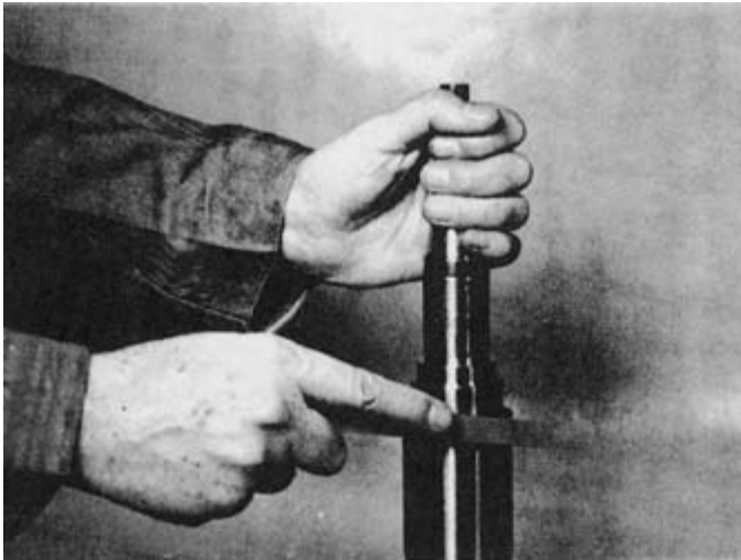
Figure 7-26. A file or stone may be used to remove nicks and burrs.
