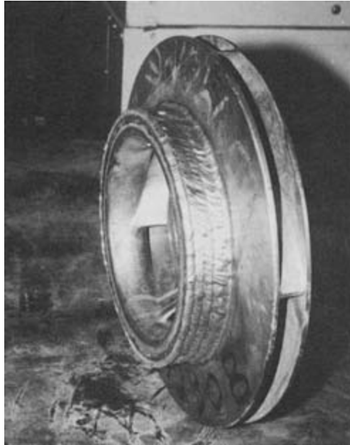
Figure 8-18. Impeller with direct overlay of Stellite to replace wear rings.
