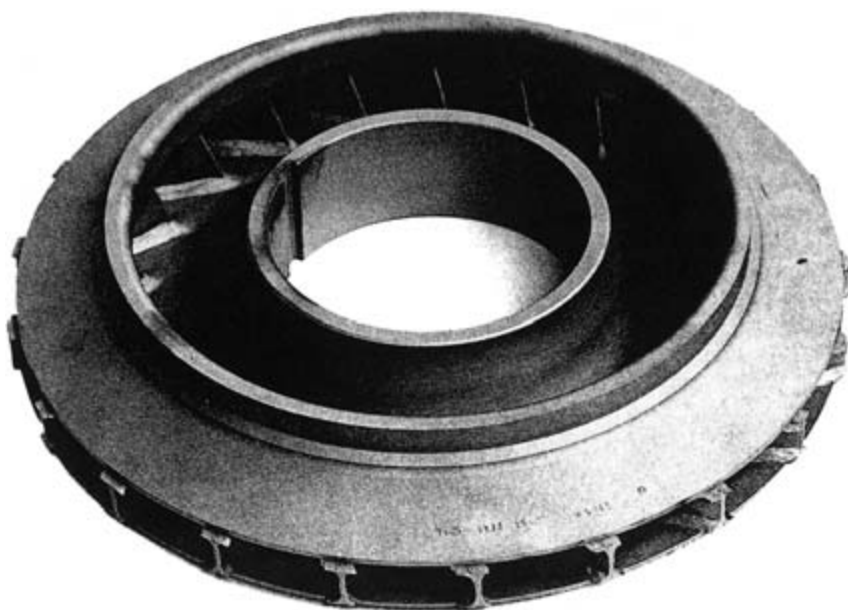
Figure 8-30. The impeller shown in Figure 8-29 after weld repair and final machining. The impeller was heat treated prior to machining and overspeed tested at 115 percent of maximum continuous speed in accordance with API specifications.
