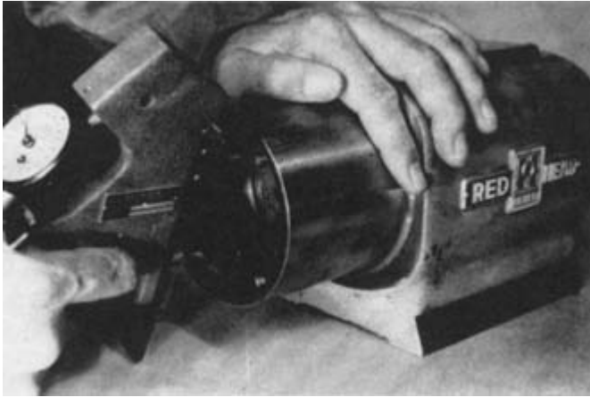
Figure 7-33. Indicator-type gauge commonly used to check housing bore dimensions.
