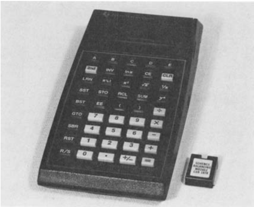
Figure 6-46. Programmable pocket calculators with balancing module make it easier and faster to determine the correction masses when field balancing.
