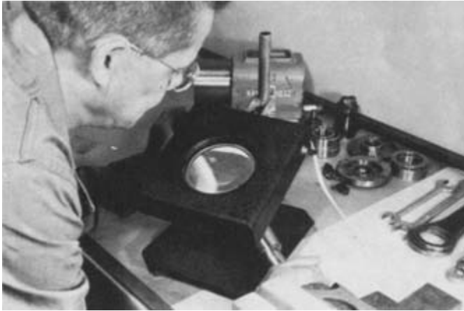
Figure 7-20. After cleaning, inspect spindle parts by visual means and under magnification. It is important that locating surfaces are free of nicks, burrs, corrosion, etc.
