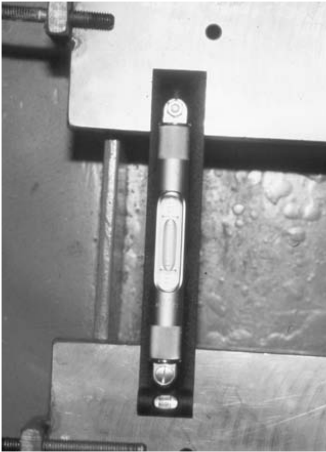
Figure 3-44. Field leveling in transverse direction.
