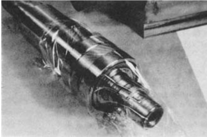
Figure 7-55. Cover subassemblies, especially those with mounted bearings, with plastic material while waiting to assemble into housing.
