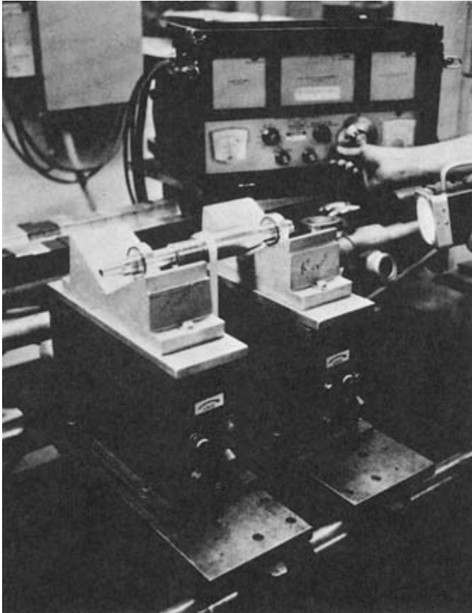
Figure 7-68. Dynamics of balancing spindle assembly. This equipment is used by TRW's Spindle Maintenance Department, but other types are available which will balance assemblies as accurately as necessary.
