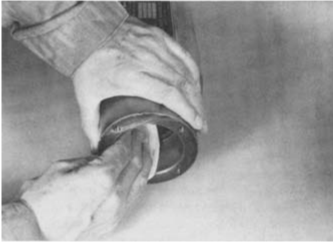
Figure 7-19. Clear bearing seats of housing thoroughly to remove all foreign matter. Then inspect bearing seats and corners for possible damage.
