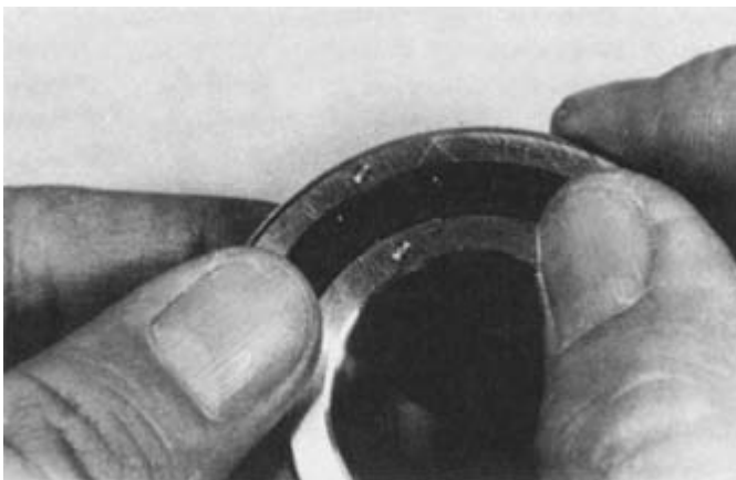
Figure 7-56. Burnished dots show high point of eccentricity.
