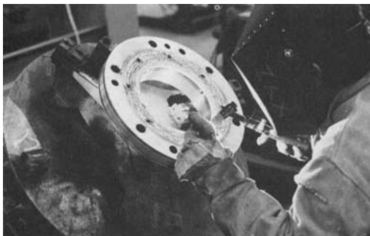
Figure 8-22. Overlaying of seal flange faces.
