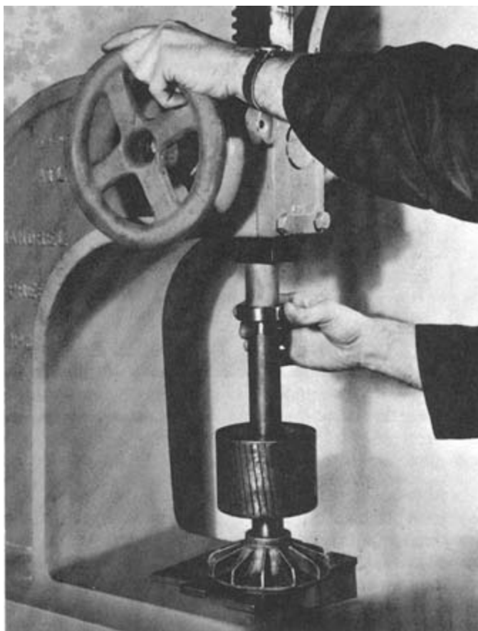
Figure 7-64. Bearing may be pressed on shaft using a tube and arbor press.
