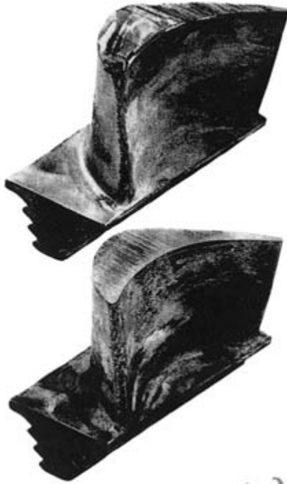
Figure 8-25. Gas expander blades of superalloy are typical examples of new parts deliveries that can exceed 10 months. These blades can be repaired with controlled welding, heat treatment, and coating processes in weeks.
