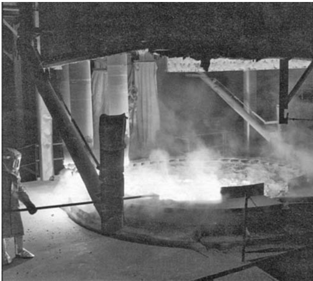
FIGURE 5.1 Higgins-type electric arc furnace for fusion processes of alumina and zirconia. (Courtesy of Saint-Gobain Abrasives. With permission.)
