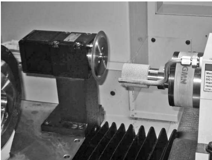
FIGURE 15.47 A postmounted dc brushless servoelectric drive dresser spindle mounted in a grinder dressing on seeded gel wheels.
