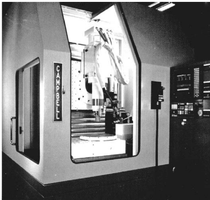
FIGURE 16.37 Example of 5-axis vertical spindle grinder for aircraft engine vane multi-surface grinding.
