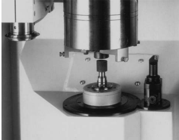
FIGURE 18.30 Combination grind and turn arrangement with part loading through the vertical workhead. (From EMAG 2001b. With permission.)
