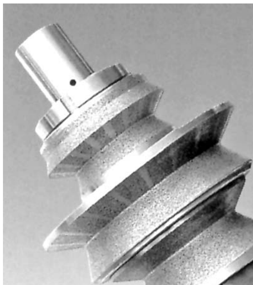
FIGURE 7.34 Diamond-free areas on shoulder of reverse-plated roll.
