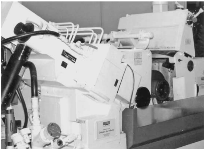
FIGURE 15.58 Rebuilt Cincinnati 220-8 centerless grinder with servo-driven plunge rotary diamond dressing.
