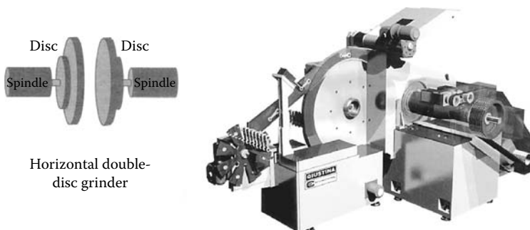
FIGURE 16.54 Horizontal spindle double-disc grinder. (Courtesy of Guistina. With permission.)
