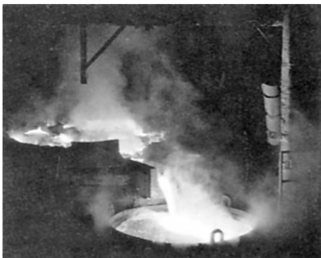
FIGURE 5.2 Pouring of molten alumina. (From Wellborn 1994. With permission.)
