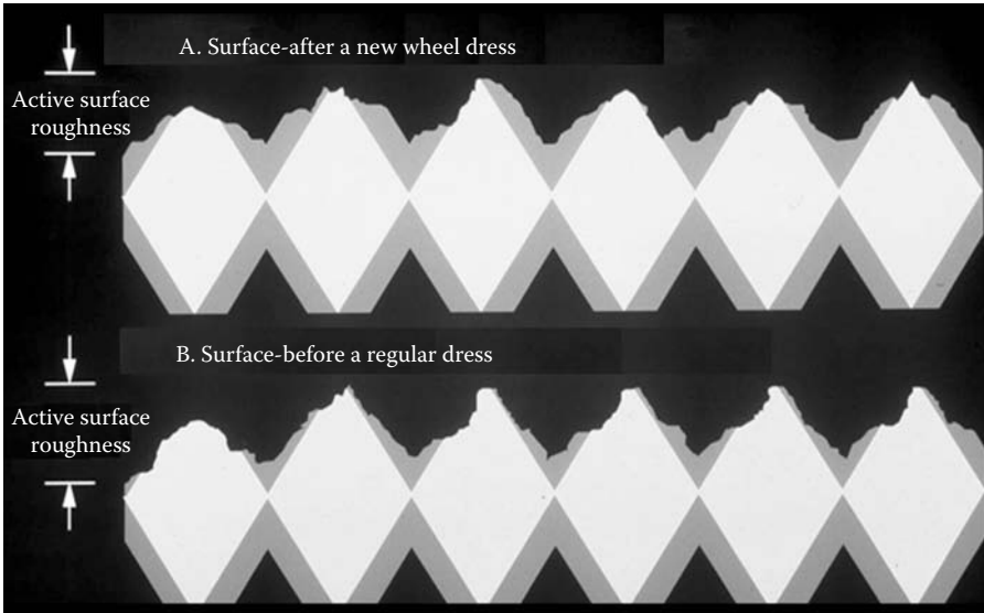
FIGURE 7.22 Concept of “active surface roughness.”
