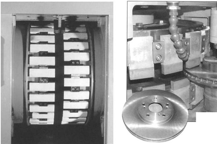
FIGURE 16.69 Examples of alox and superabrasive stone grinding of brake rotor discs. (From Daishi 2001, Thielenhaus n.d. With permission.)
