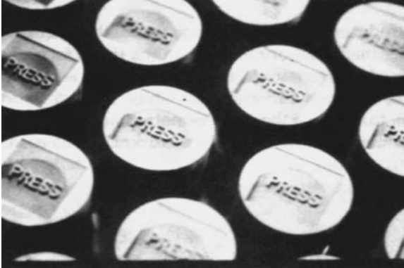
Figure 2.15 Graphite EDM electrodes machined by USM (Gilmore, 1995).
