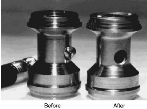
Figure 4.33 EC deburring applications ( www.extrudehone.com/cation ).
