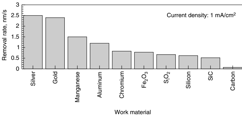
Figure 5.59 Variation removal rate with work material in IBM (El-Hofy, 1995).
