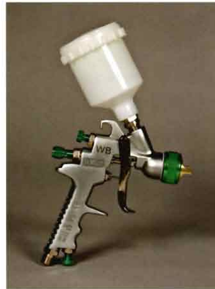
Gravity guns have the cup mounted on the top. They come in full-size guns as well as small detail guns like this one holding about 4 oz. of finish.
