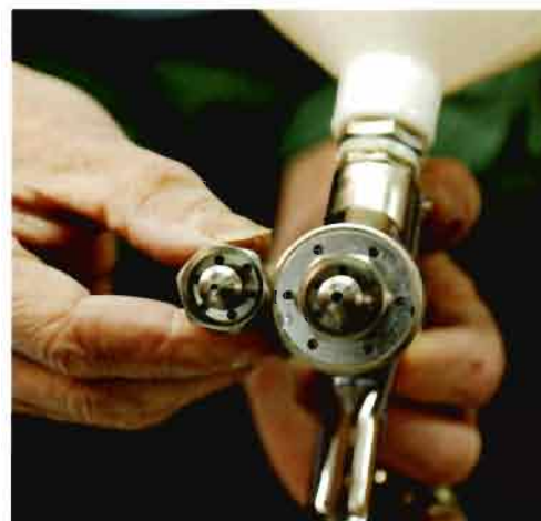
A 2.5 mm nozzle that's installed in this gravity gun is much larger than ones used for clear finishes. A 1.6 mm is held next to it for comparison. Don't even try to spray latex with a small nozzle.
