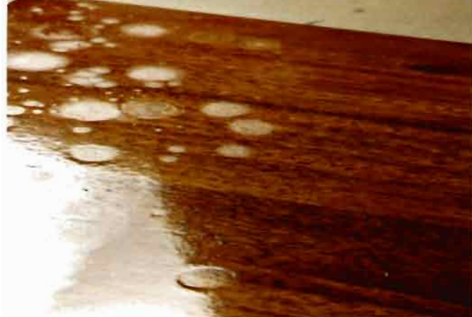
Sometimes fish-eye looks a little like orange peel, but it's random. Note that the right side of the panel isn't affected.
