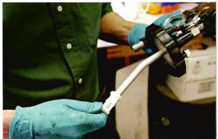
A gun strainer for a bottom-cup gun.
