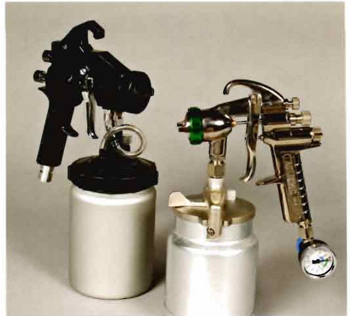
Siphon cups can run off a turbine (left) or a compressor. The turbine guns are always pressurized, while the compressor-driven versions can be pressurized or suction feed like the one shown.
