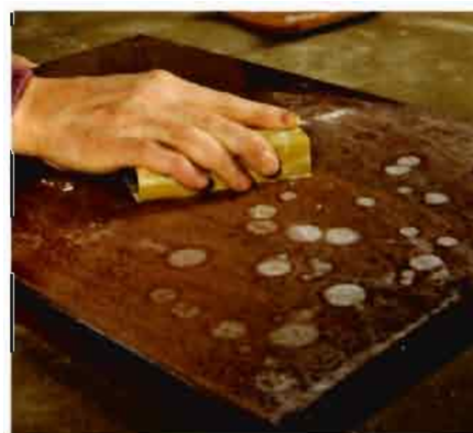
To remove fish-eye that's dried, sand the finish level with sandpaper.
