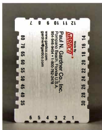
A wet-mil gauge. Use the side numbered 1 to 6.
