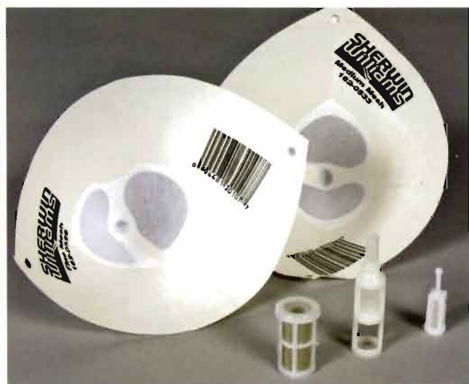
Paper cone strainers are sold in fine, medium, and coarse grades. The fine and medium ones shown here work with all paints, stains and clear finishes. The in-gun strainers shown in front are installed somewhere in the spray gun. Ideally you should use both.
