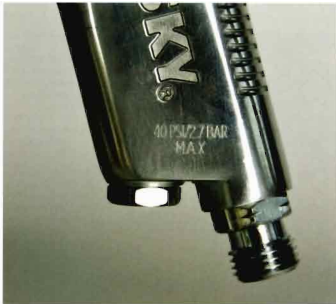
HVLP compressor-driven spray guns indicate the maximum inlet pressure near the air inlet. Running the gun at this pressure produces 10 psi air cap pressure (the maximum pressure allowed for HVLP) at the point where the finish comes out the front.
