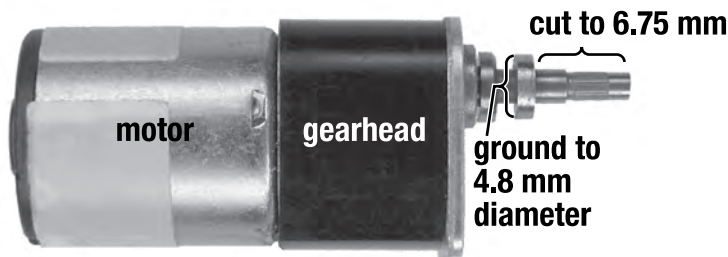
Figure 18-18. Specifications for the Nihon gearmotor shaft after being altered to reduce the shaft length and diameter
