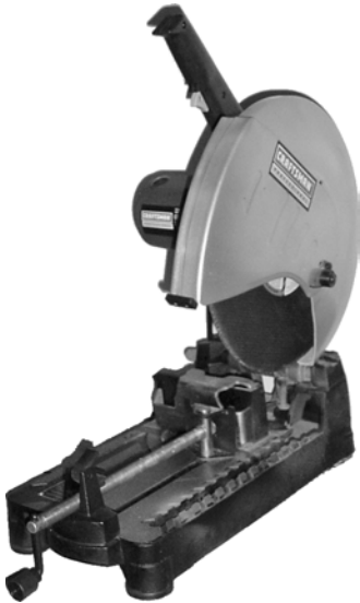
Figure 1-3. A large, abrasive cutoff disc machine for cutting lengths of raw material faster and straighter than using a hacksaw
