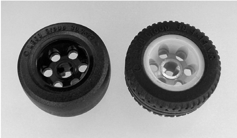
Figure 18-23. Slippery LEGO front wheel (left) and grippy LEGO rear wheel (right)
