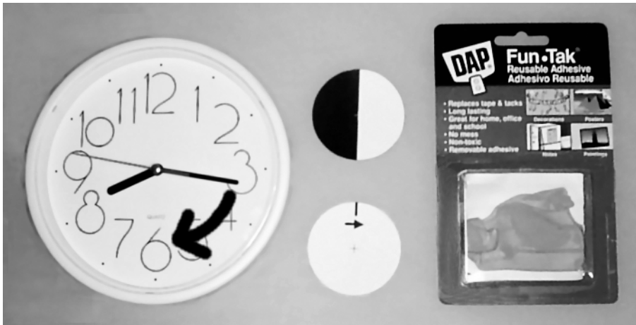
Figure 9-2. Clockwise is the direction that clock hands travel, as viewed when the motor's shaft points toward you (left). Two example target discs for attaching to a motor shaft to observe direction of rotation (center). The top disc is more reliable for electronic tachometers or counters. The bottom disc is easier for humans to count rotations or detect the direction of rotation. Reusable, moldable adhesive (such as stretchy modeling clay) makes it easy to temporarily attach a disc to a motor shaft for testing (right).
