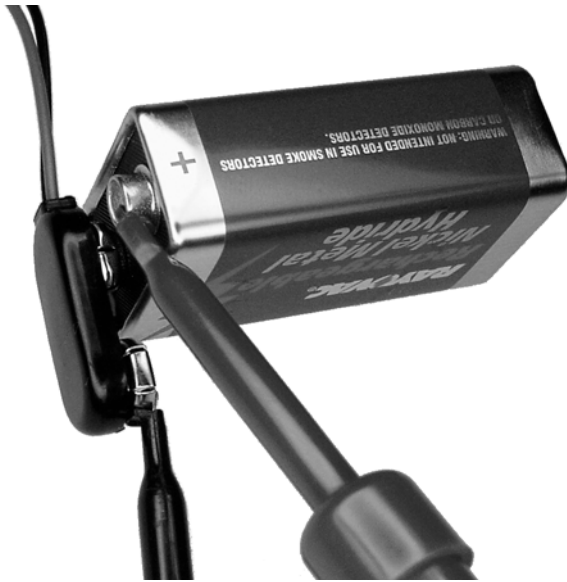
Figure 14-2. Connecting a multimeter between one battery terminal and the battery snap to measure current
