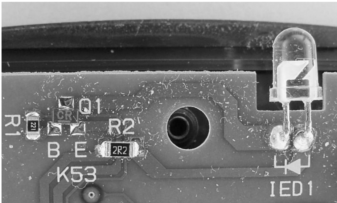
Figure 11-12. The inside of a standard consumer remote control. Resistor R2 is labeled “2R2,” which is a resistance of 2.2 \Omega . With two fresh AA batteries supplying 3.2 V, assuming a 1.2 V drop across IED1 and a 0.2 V drop across the bipolar transistor driver, the infrared LED receives current pulses of 0.81 amp.
