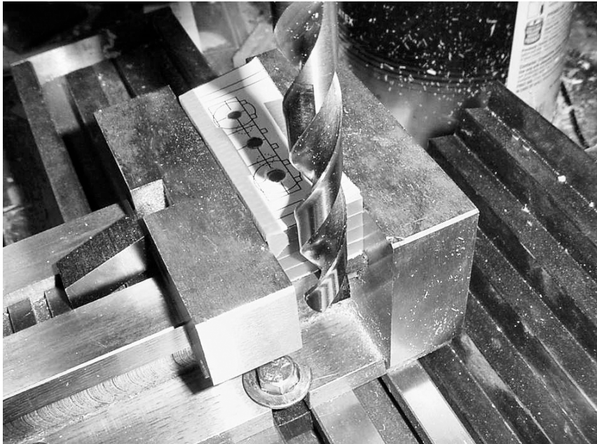
Figure 13-31. Setting the limit block for the new depth of the longer drill to avoid drilling into the vise. Notice that in this picture the stack has three \frac{3}{16} -inch diameter holes drilled in it as described in the prior instructions. Also notice that although tape is being used to hold the paper template onto the top of the stack, each workpiece is being held firmly in place by the vise (not merely by tape).
