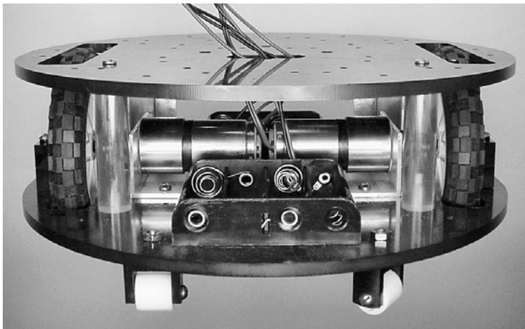
Figure 18-5. Roundabout Pro's body features a lot of space for robot parts by connecting two platforms together. You can mount battery packs, circuit boards, and sensors above and below each platform.
