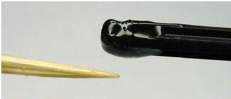
Figure 4-8. A notched LEGO cross axle coated with epoxy, ready to be inserted into the coupler. You can use a toothpick to nudge the epoxy into the grooves in the cross axle.
