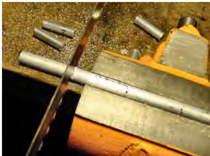
Figure 3-2. Hacksaw cutting lengths of solid aluminum rod gripped in vise. By the way, I'm left-handed. Those of you who are right-handed may want to extend the workpiece over the right side of the vise for cutting.
