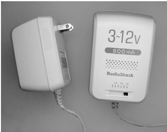
Figure 6-9. A consumer-adjustable AC adapter provides regulated 3 V, 4.5 V, 6 V, 7.5 V, 9 V, or 12 V with up to 800 mA of current.
