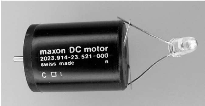
Figure 9-3. A plain (non-gearhead) motor with an LED across the terminals to demonstrate where the energy is going in a fast-decay setup
