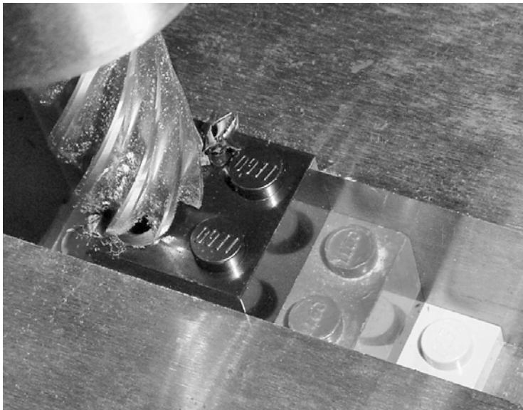
Figure 17-17. Milling off the top posts of a LEGO brick. Place additional LEGO bricks underneath in the vise to secure, level, and raise the top brick to the proper height.
