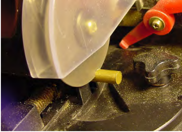
Figure 3-3. A small cutoff machine with built-in V-groove vise ($139.95, #15218 at Micro-Mark) cuts rod smoothly and at the proper angle so that sanding or filing may not be necessary. Larger machines are available at local hardware stores.
