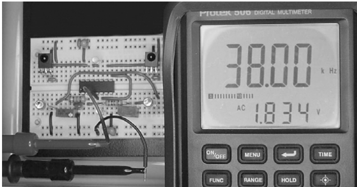
Figure 12-3. A multimeter with a frequency measurement mode is probably the best way to tune the circuit.
