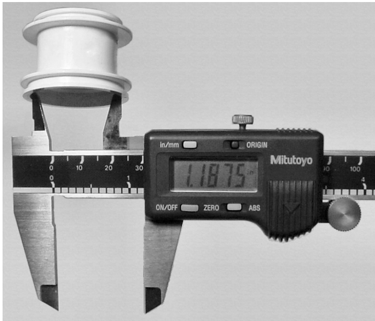
Figure 5-6. Measuring the internal diameter of the outside of a LEGO 49.6 by 28 VR wheel hub using digital calipers
