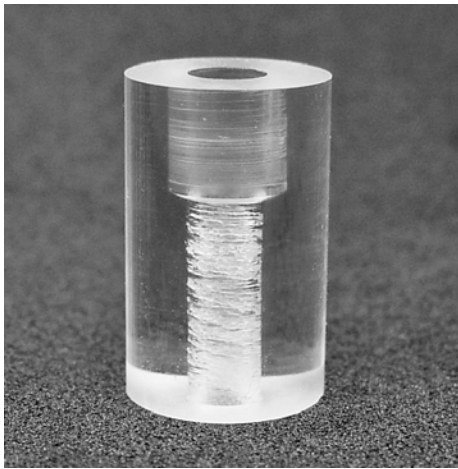
Figure 2-4. Desirable: Coupler with nicely centered, straight-angled holes
