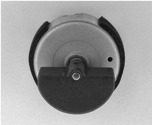
Figure 2-6. A motor with a heavy, offset mass causes vibrations when spun. (This motor was removed from a "force feedback" joystick.)
