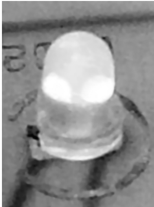
Figure 14-4. A two-lead bicolor LED with both dies illuminated “simultaneously” by rapidly switching the polarity back and forth
