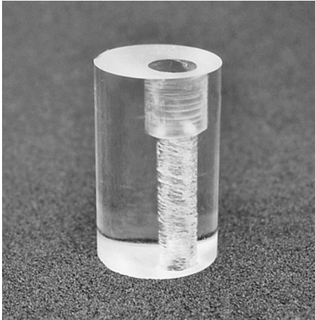
Figure 2-5. Permissible: Although each hole is nicely centered with respect to the other and they have nice, straight, parallel alignment, the holes aren't centered within the coupler body itself.
