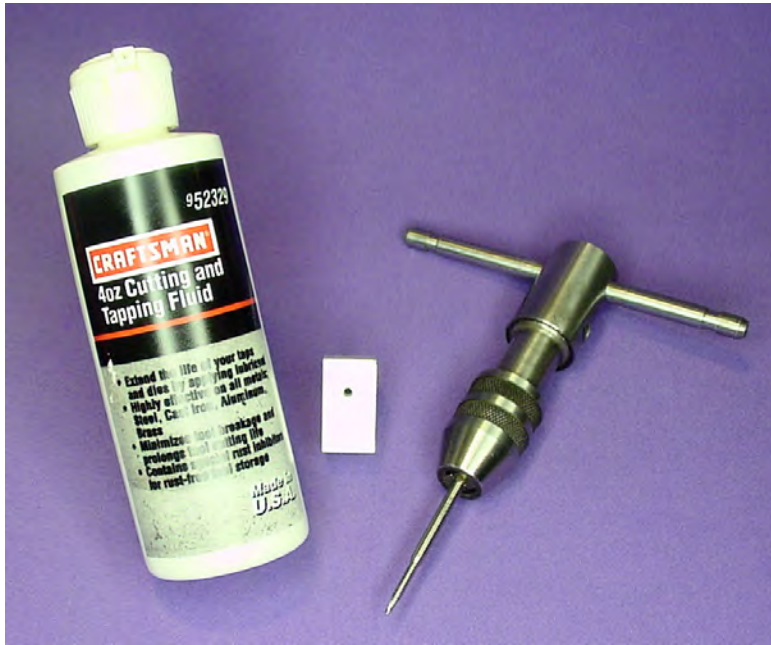
Figure 3-13. Tapping fluid, coupler fixture with setscrew hole drilled in it, and tap wrench with #4-40 tap (left to right)
