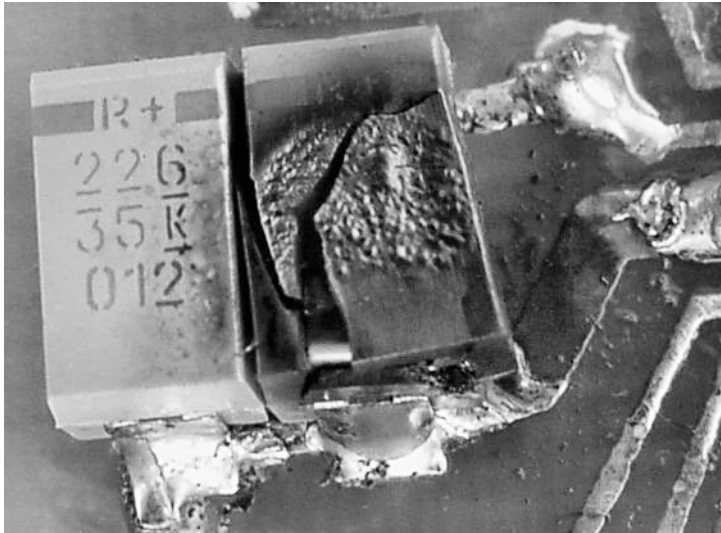
Figure 8-5. A bulk unregulated tantalum capacitor exploded and caught fire on the Soup robot.
