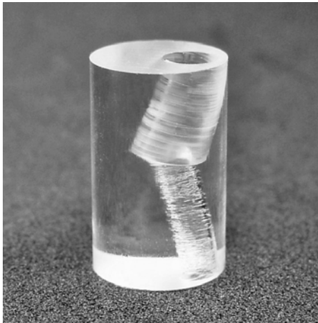
Figure 2-9. Avoid like the plague: Although the holes are somewhat centered over each other, the angles are horribly different.
