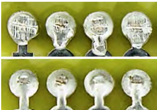
Figure 16-13. Solder joints before reheating (top). Those same solder joints after reheating (bottom).
