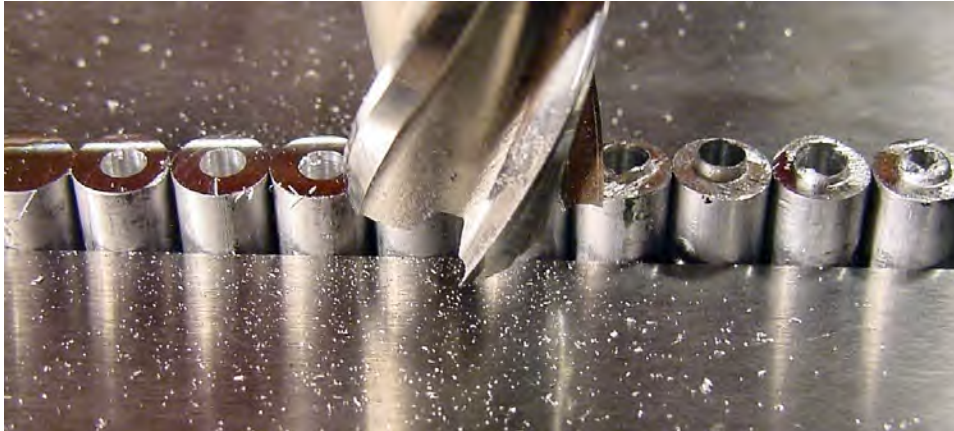
Figure 3-6. A vertical milling machine smoothly cutting the tops of the rods. Note that in this picture, the shaft holes have already been drilled in the coupler bodies. This is because I'll often cut the rods smooth both before drilling and after drilling.
