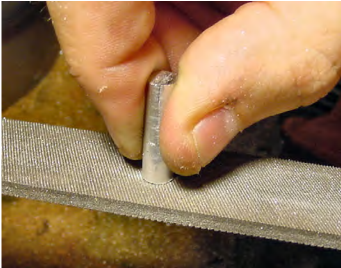
Figure 3-4. Filing smooth the edges of the cut rod by holding the rod piece in one hand and drawing it across the file, which is held in the other hand. What? No! That's not how you're supposed to file!
