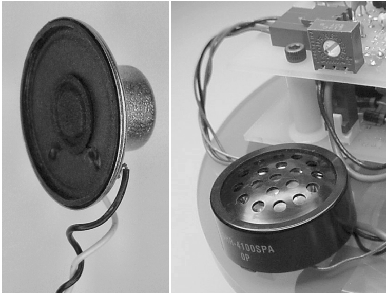
Figure 18-2. An ordinary 8 \Omega speaker removed from a discarded personal computer (left). A compact speaker with protective cover that's glued to a piece of plastic and screwed in from underneath (right). Note the square trimpot (R5) at the top right of the picture, which adjusts the volume.
