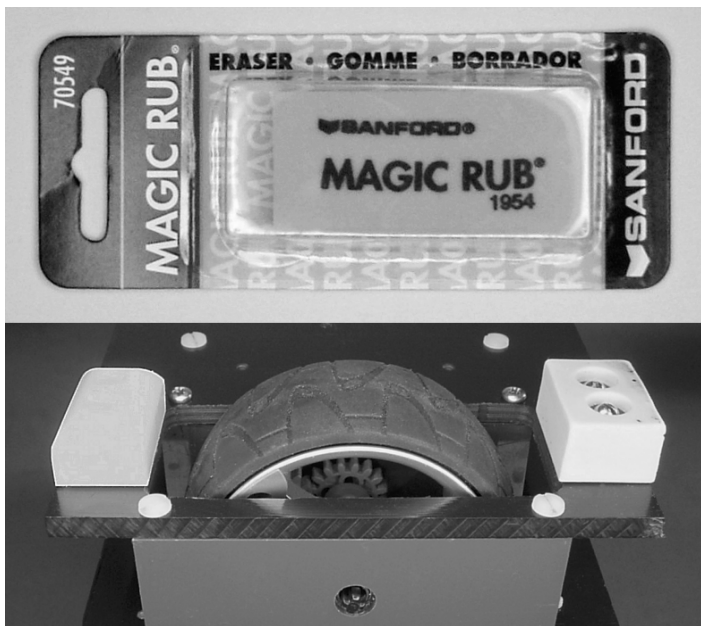
Figure 13-36. Soup, which uses the same type of motor mounts as Roundabout, has chamfered slick Teflon slides in the rear and high-friction erasers in the front. Notice the screw holes in the center of the eraser (lower right) for securing the eraser to the robot's body with screws and washers.
