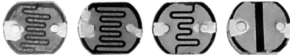
Figure 17-2. Different gap or grid patterns. Given the same photoconductive base material, the leftmost pattern (narrow and wavy) provides a lower resistance but lower permitted voltage. The rightmost pattern (wide and straight) provides a higher permitted voltage but also a higher resistance.
