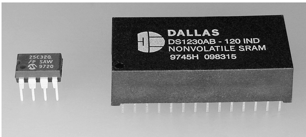
Figure 15-10. External nonvolatile memory. A 25C320 32 Kb SPI-serial EEPROM (left). The 24xxx series is available for I 2 C and 2-wire serial access. The 93xxx series is available for three-wire serial access. A DS1230 256 Kb parallel SRAM with built-in lithium battery backup (right). This has the high-speed and unlimited-write benefits of volatile memory, yet the memory contents are retained for up to ten years without power.
