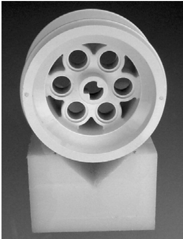
Figure 5-22. A V-block partially surrounds a cylindrical object and holds it at two points to prevent it from popping out of a vise during machining.
