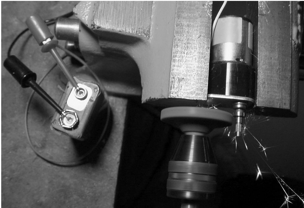
Figure 18-19. Grinding down the wide portion of the shaft with a Dremel grinding stone accessory. The gearmotor is powered by a rechargeable 9 V battery (about 7.2 V) to rotate the motor shaft during grinding to ensure the reduction is even all of the way around. The grinding process produces spectacular sparks.
