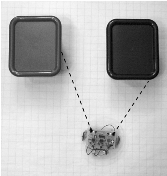
Figure 14-8. A lighter-colored object (in this case, red) on the left side reflects an equal amount of infrared light as does the nearer but darker-colored object (in this case, blue) on the right side. In this figure, Roundabout isn't moving because it senses 50 percent detection on both sensors. Therefore, both motors are driven backward and forward very quickly, resulting in no overall movement.
