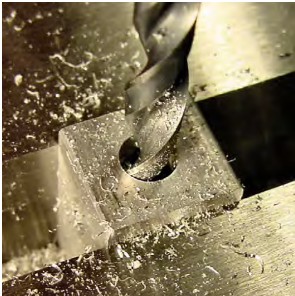
Figure 3-19. Drilling the coupler rod hole
