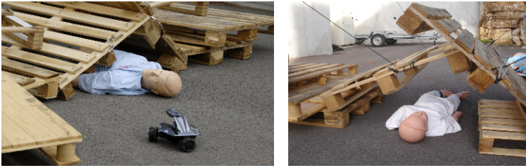
Fig. 5 MARIONET-CRANE used from freeing a victim from rumbles.
