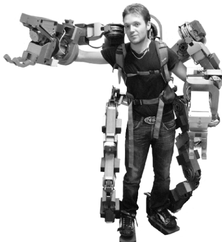
Fig. 1 Fully actuated body extender developed at PERCRO.
