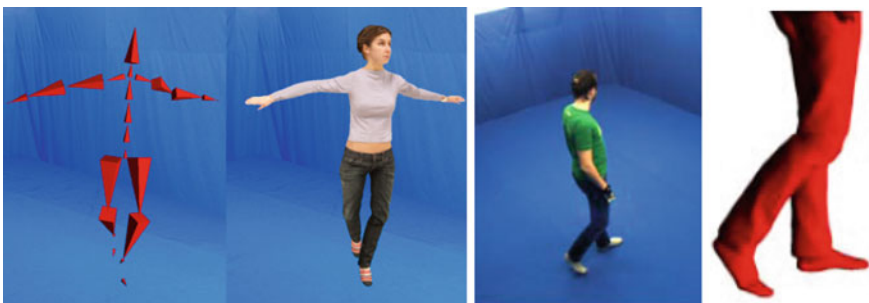
Fig. 3.7 Markerless motion capture of skinned models: a textured deformable mesh with skeleton is driven by silhouette information and optical flow features in a four cameras setup (image courtesy of [15])
