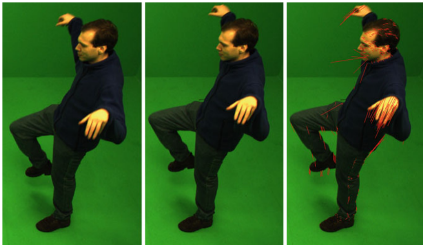
Fig. 4.26 SIFT temporal matching: Source image at t (left), target image at t + 1 for the same camera (middle), and the resulting estimated set of sparse SIFT features between the two consecutive frames (right)
