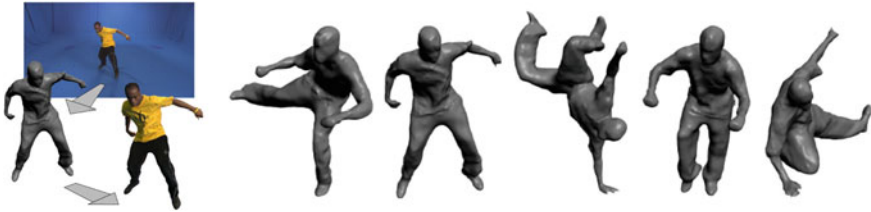
Fig. 3.3 Surface performance capture: surface capture of a hiphop dancer is recorded in a dedicated chroma-key blue-screen studio with 8 HD Thomson Viper cameras. At each frame, a temporal independent close polygonal model with small-scale surface details is generated as output of the system (image courtesy of [8])
