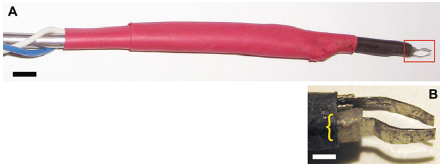
Fig. 2 Custom platinum electrode. (a) The plates of the electrode are constructed out of platinum foil that is soldered to insulated wire leads. The plates are isolated from one another with shrink tubing. A larger piece of shrink tubing holds the aligned plates in place, and a still larger piece of shrink tubing holds the electrode onto the rod that fits in the micromanipulator. Scale bar=5 mm. (b) A magnified view of the tip of the electrode showing the folded platinum foil that is folded and cut into ~1 mm wide plates. The bracket indicates the shrink tubing that insulates electrodes from one another. Scale bar=2 mm
