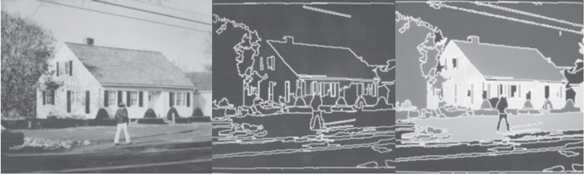
FIGURE 1-3. Segmentation of a scene into candidate regions provides the bridge between the original image and the interpretation of a scene in VISIONS by associating regions of the image with schema instances. In this example, VISIONS classifies regions of the scene as sky, roof, wall, shutter, foliage, and grass, but it leaves other areas uninterpreted. (Figures supplied by kind courtesy of Allen Hanson.) (See color insert for full color version of this figure.)
