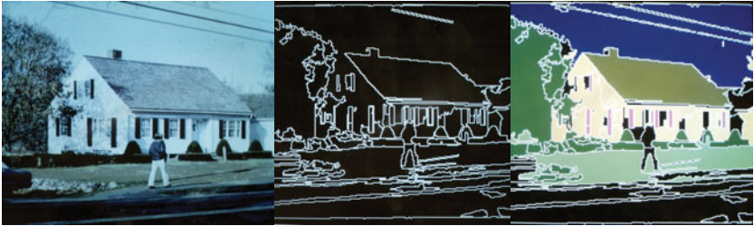
FIGURE 1-3. Segmentation of a scene into candidate regions provides the bridge between the original image and the interpretation of a scene in VISIONS by associating regions of the image with schema instances. In this example, VISIONS classifies regions of the scene as sky, roof, wall, shutter, foliage, and grass, but it leaves other areas uninterpreted. (Figures supplied by kind courtesy of Allen Hanson.)
