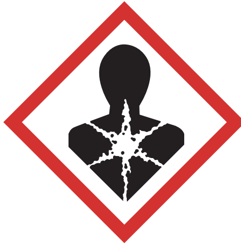
Figure 14-17. Warning symbol for respiratory sensitization, cancer, and other human health hazards. This symbol, with the diamond shape, is part of the Globally Harmonized System of Classification and Labeling of Chemicals.
