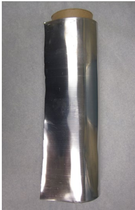
Fig. 8 Lead roll 0.762 mm thickness used to make shields
