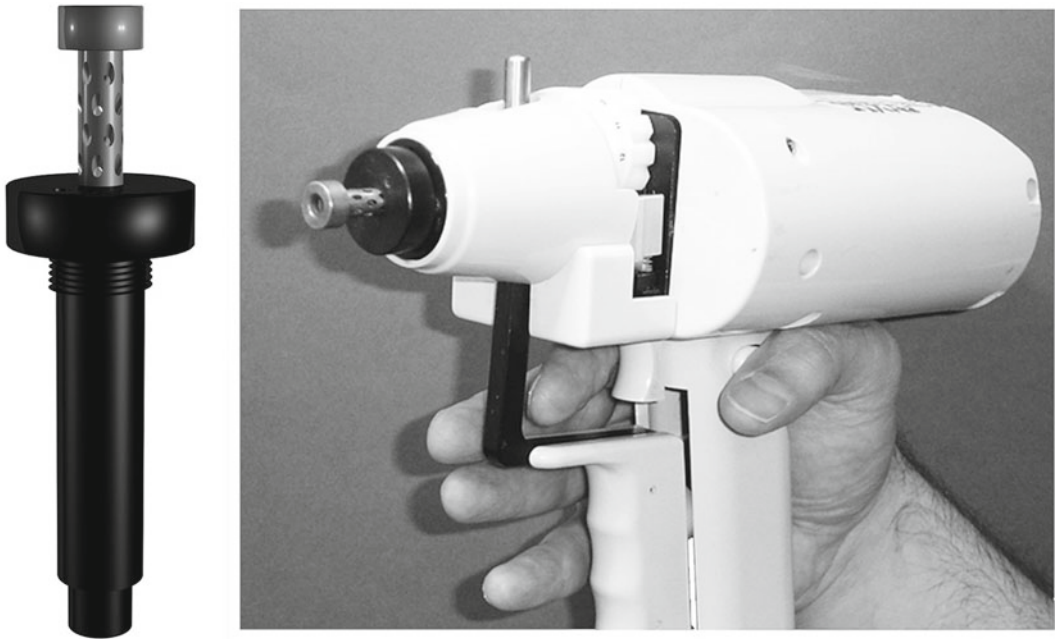
Fig. 3. The Bio-Rad gene gun and the modified gene gun barrel that can be easily attached to the gene gun.
