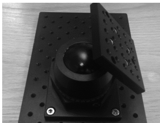
Figure 3. The sample/mask plate holder with rotation features for multi-directional inclined UV exposure.
