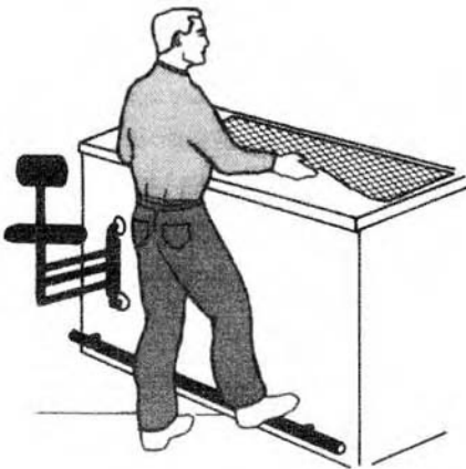
FIGURE 30.3 Bar footrests along a work station or conveyor can reduce standing stress. (From Rodgers, S. 1984. Working with Backache . Perinton Press, Fairport, NY. With permission.) A small platform is another alternative. (From Konz, S. and Johnson, S. 2004. Work Design: Occupational Ergonomics , 6th ed. Holcomb-Hathaway, Scottsdale, AZ. With permission.)
