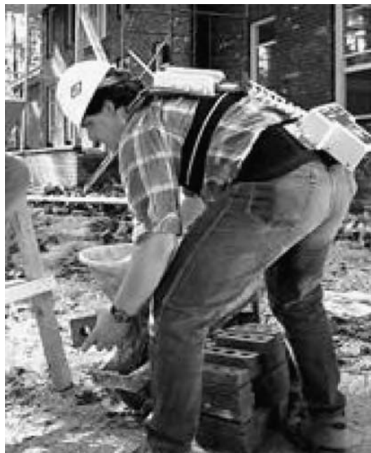
FIGURE 35.1 The Lumbar Motion Monitor.
