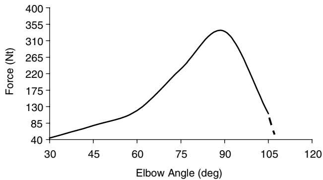
FIGURE 11.6 Position-force diagram produced by flexion of the forearm in pronation. “Angle” refers to included angle between the longitudinal axes of the forearm and upper arm. The highest parts of the curve indicate the configurations where the biomechanical lever system is most effective. (Adapted from Chaffin, D.B. and Andersson, G.B., Occupational Biomechanics , John Wiley & Sons, Inc. New York, 1991. With permission.)
