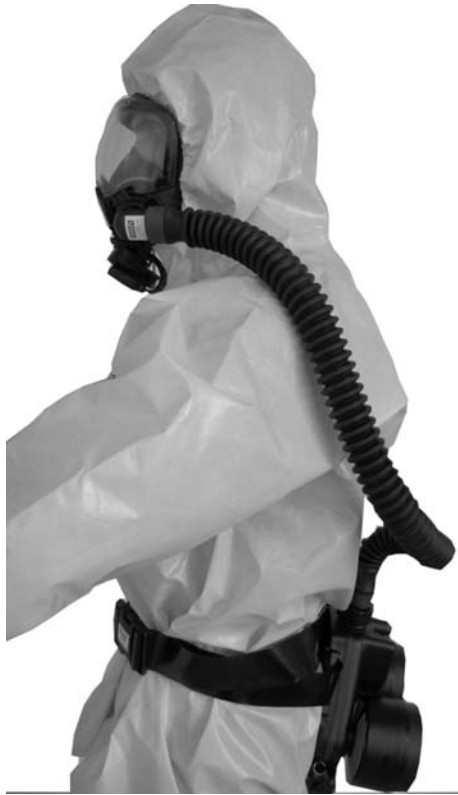
FIGURE 5-8 Powered air-purifying respirator with tight-fitting facepiece worn with a disposable suit; a blower with canisters is worn on the waist, with the air supply hose leading to the facepiece.
