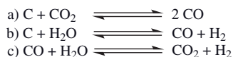
Scheme 11.5 Important equilibrium reactions in gasification; (a) Boudouard equilibrium; (b) Water gas reaction; (c) Shift reaction.
