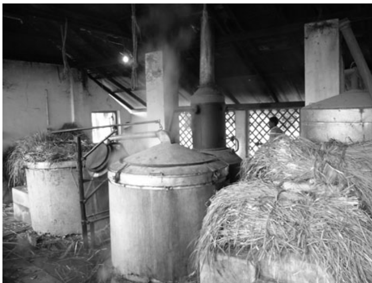
Fig. 18.8 Boiler and distillation chamber of steam distillation unit.
