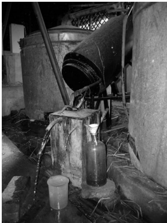
Fig. 18.9 Condenser and oil separator of steam distillation unit.
