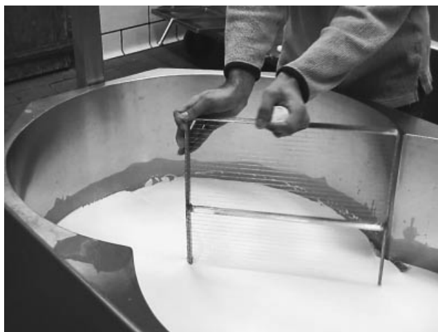
Figure 11.2. Cutting of rennet curd.
