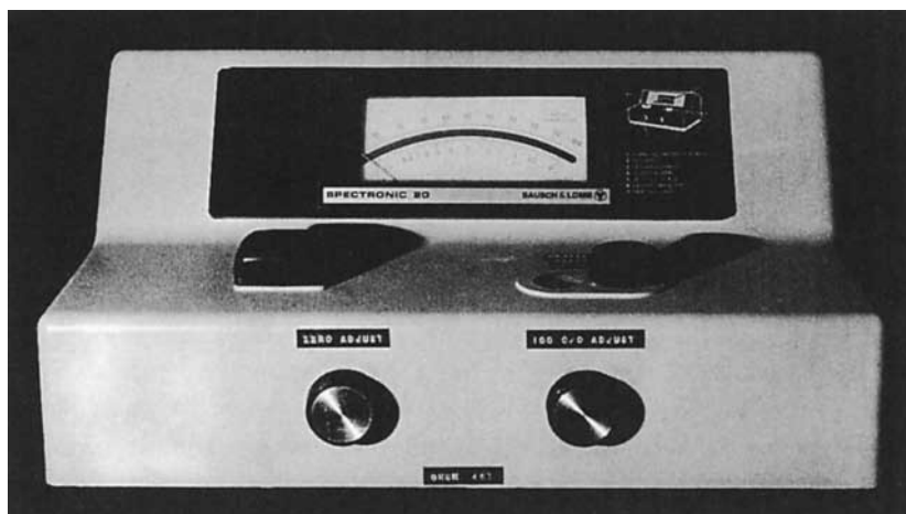
Figure IV.6 A Spectronic 20 spectrophotometer. The absorbance of a solution can be reliably read to within about 1%. (Sherman Schultz)
