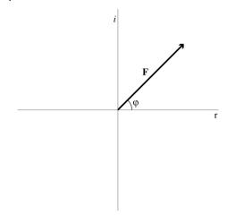
**Figure 2.7** Argand diagram showing the vector representation of a wave. The real and imaginary axes are horizontal and vertical, respectively. The magnitude of the wave is represented by the magnitude of the vector  $|\mathbf{F}|$  and the phase by  $\varphi$ . Here, the phase of the wave is 45° or 0.125 cycles.
