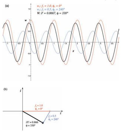
**Figure 2.8** Summation of waves. (a) Summation of waves 1 (red) and 2 (blue) to the combined wave shown in black. The amplitude and phase parameters of the waves are listed. The wavelength for all waves are the same (1.0).
