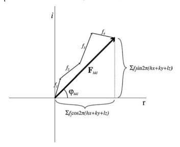
**Figure 2.15** Argand diagram illustrating a structure factor for the single reflection, *hkl*, from a unit cell consisting of four known atoms. This assumes the atomic coordinates are known for the four atoms to draw the individual scattering factors with known magnitude and direction.
