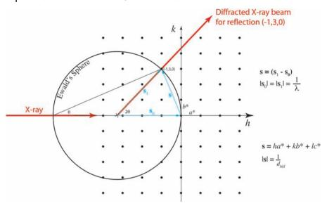
**Figure 2.14** Bragg's law in reciprocal space. Shown is reciprocal space lattice from Figure 2.11. Drawn on the lattice is Ewald's sphere of reflection with a radius of  $1/\lambda$  (x marks the center of sphere). The vector **s** can be defined in general by  $ha^* + kb^* + lc^*$ , where  $a^*$ ,
