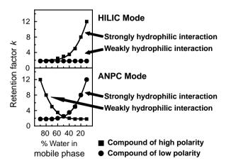
**Figure 5.4** Scenarios for the HILIC retention mode and the ANPC retention mode for the separation of compounds of different hydrophilicities. The top plot (called Figure 5.4(a) in the text) refers to the HILIC mode, whilst the bottom plot (called Figure 5.4(b) in the text) refers to the ANPC mode.
