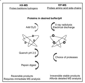
Scheme 1.1 Experimental procedures for HX-MS and RP-MS.
