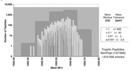
**Figure 1.3** Role of high mass accuracy in reducing false-positives from database searches. This histogram (from [23]) shows the number of tryptic peptides at different mass accuracies for a 1996 GenPept database. For a nominal molecular weight of 1000, there are around 5000 tryptic peptides if the measurements are accurate to 0.5 Da
