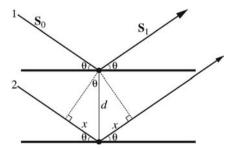
**Figure 2.12** Scattering of X-rays off two parallel planes. Two planes with an interplane spacing of *d* contain point scatterers above each other. Wave 2 scattered from the bottom plane must travel an extra distance  $(2 \times)$  than wave 1 from the top. If the scattered waves are in
