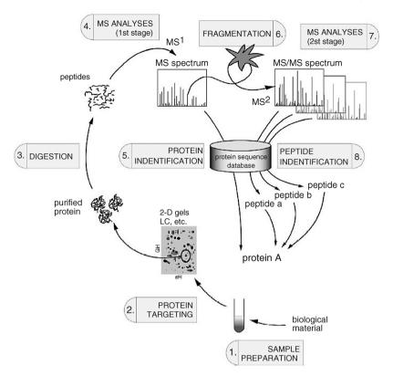
**Figure 14.1** Typical workflow for "bottom-up" protein identification. The first steps (1) and (2) are preparing the sample and targeting proteins to analyze. Then the proteins are digested (3) and the resulting peptides undergo MS analysis (4) yielding an MS spectrum that can be identified by an MS identification algorithm (5). The analysis can go further
