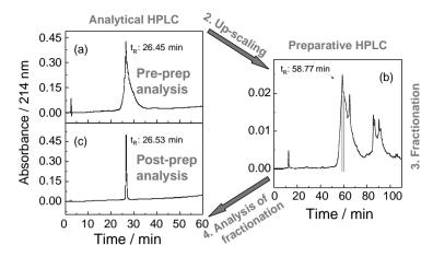
**Figure 5.7** Prepreparative analysis (a), preparative fractionation (b), and postpreparative analysis (c) with HP-RPC for the preparative isolation of synthetic polypeptides NH<sub>2</sub>-RIC(Acm)DKC(Acm)KVIRRHGRVYVIC (Acm)ENPKHKQ-COOH [114]. The prepreparative analysis of crude synthetic polypeptide (a) and postpreparative analysis of the purified product (c) was achieved with a TSK-ODS-120 T column (4.6  $\times$  150 mm ID,
