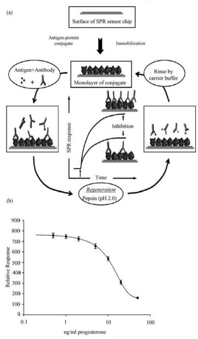
**Figure 7.6** (a) Schematic view of the indirect competitive inhibition SPR immunoassay. (b) RU response versus concentration of progesterone in bovine milk – a standard curve. Reprinted from [17, 101], with permission from Elsevier.
