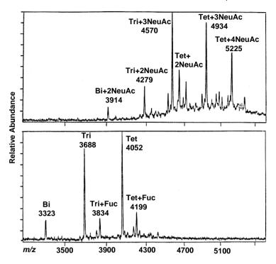
Figure 1.7 Negative-ion MALDI-TOF mass spectra displaying carbohydrate heterogeneity (bi-, tri-, and tetra-antennary) for glycopeptide site III (IQATFFYFTPN\*KTE) obtained from Staph V8 digest of human  $\alpha_1$ -acid glycoprotein; (top) before and (bottom) after treatment with
