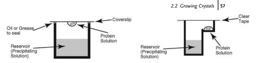
**Figure 2.1** Schematic illustration of vapor diffusion crystallization setups. Left shows the typical "hanging drop" experiment where around 1–5  $\mu$ l of protein solution is suspended on a glass coverslip over around 1 ml reservoir
