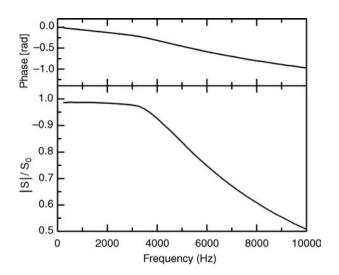
**Figure 8.10** Calculated describing function (transfer function for nonlinear systems) of the tapping mode AFM probe in air for 40 N/m spring constant, 250 kHz resonance frequency,
