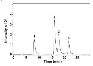
Figure 5.5 Aqueous normal-phase separation of polar peptides. Column: silica hydride Diamond from Higgins Analytical  $(0.30 \times 150 \text{ mm}, 4 \text{ mm})$ ; peptides: (1) Asp-Ala, (2) Arg-Gly-Asp, (3) Gly-Gly-His, (4) Gly-Arg-Ala-Asp-Ser-Pro-Ly s; eluent A: 0.1% formic acid in
