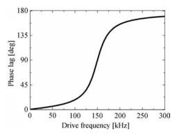
Figure 8.2 Example of a phase resonance curve, based on Eq. (8.4).
