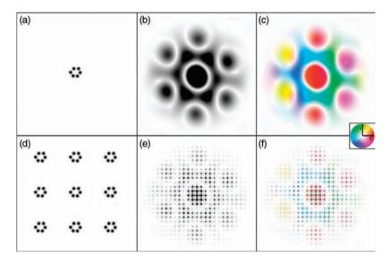
**Figure 2.13** Illustration of X-ray scattering from a single motif and a crystal lattice of the motif. Top panels show the motif in (a), recorded X-ray scattering pattern only showing intensities in (b) and the scattering pattern with phase information in (c). The bottom panels
