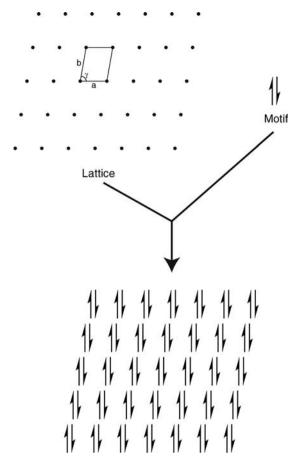
**Figure 2.3** Illustration of crystal (bottom) being composed of a motif (top right) repeated in a lattice (top left). One two-dimensional unit cell is outlined in the lattice.
