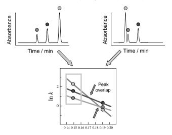
**Figure 5.6** Optimization of isocratic elution. Two chromatograms obtained for 19 and 14% (v/v) of organic solvent modifier in the mobile phase (corresponding to  $\varphi = 0.19$  and 0.14, respectively) can be used to plot the resulting
