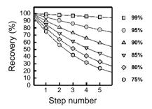
**Figure 5.8** Overall recovery at a fixed recovery per step value with an increased number of additional steps in multidimensional chromatography.
