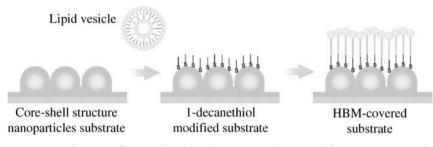
**Figure 6.4** Fabrication of the membrane-based sensor using the core–shell structure nanoparticle substrate.
