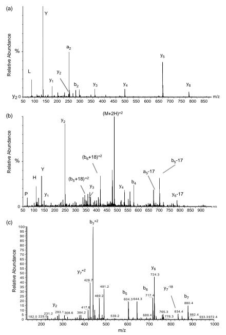
**Figure 1.5** Effect of arginine on fragment ion formation. (a) CID of  $(M + H)^{2+}$  precursor ion of the tryptic peptide YLYEIAR, where one of the protons is "mobile" and induces a contiguous series of y-type ions plus some *b*-type ions. (b) CID of  $(M + H)^{2+}$  precursor ion of the peptide YSRRHPE, which has two arginine residues and therefore no "mobile" proton.
