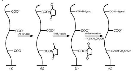
**Figure 7.5** Amine coupling of a ligand to a sensor surface. (a) Nonactivated carboxyl groups on dextran. (b) The carboxyl groups are activated by addition of a mixture of succinimide (NHS) and carbodiimide (EDC). (c) The ligand
