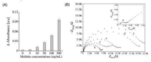
Figure 6.6 (A) Calibration curves for melittin on the membrane-based sensor using LSPR. (B) Impedance plots of the core–shell structure nanoparticle substrate (a), thiol-modified
