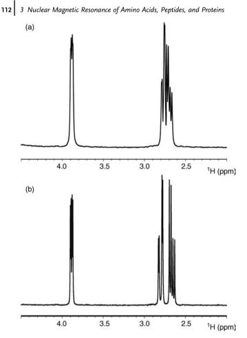
**Figure 3.3** NMR <sup>1</sup>H one-dimensional spectra of an aspartyl residue acquired at 90 (a) and 400 MHz (b). Signal resolution improvement in (b) is apparent.
