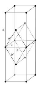
**Figure 2.4** Two cells of a C-centered orthorhombic cell outlined with solid lines. Also shown is the lower symmetry triclinic primitive cell outlined with dashed lines. The primitive a' and b' axes are labeled, with the c axis coincident with the orthorhombic cell.
