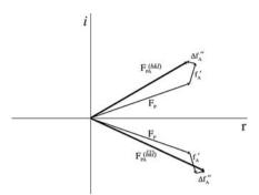
**Figure 2.17** Argand diagram showing the breakdown of Friedel's law with an anomalous scattering heavy atom. The vectors below the real axis show the components of Friedel's law for (-h, -k, -l). The structure factor for
