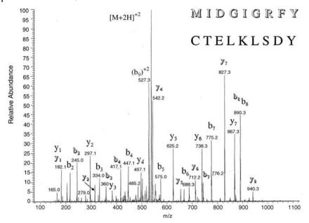
**Figure 1.9** Simultaneous CID of  $(M + H)^{2+}$  precursor ion containing two isobaric peptides with sequences of MIDGIGRFY and CTELKLSDY recorded on an ion-trap mass
