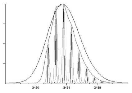
**Figure 1.2** Effect of mass spectrometric resolution on peak shape. Shown are the calculated peak shapes for the  $(M + H)^+$  ion of porcine glucagon (monoisotopic mass of 3481.62 Da and average mass of 3483.8 Da)
