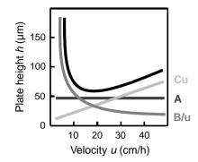
**Figure 5.3** Van Deemter–Knox plot (top curve) and plots of individual terms of the van Deemter–Knox equation: the A-term, which expresses the eddy diffusion and mobile phase mass transfer effects; the *B*-term, which
