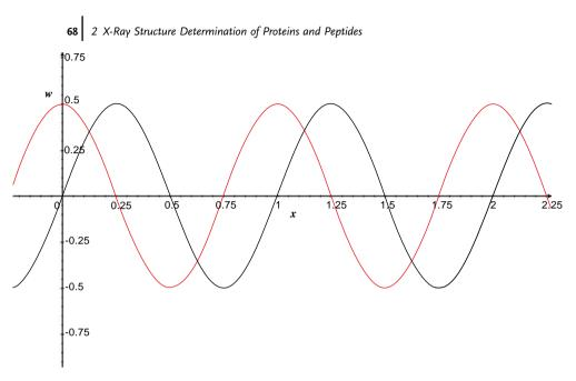
**Figure 2.6** Plot of two waves, the reference wave in red with an amplitude (*f*) equal to 0.5 and a wavelength ( $\lambda$ ) of 1.0. The black curve represents a wave with the same amplitude and wavelength as the reference wave, but shifted along *x* by 0.25 of a unit ( $x_1$  in Eq. (2.5)).
