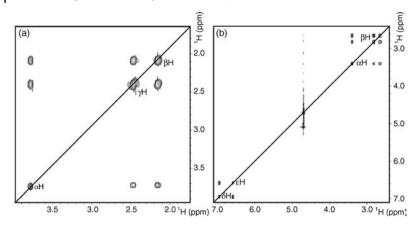
Figure 3.1 Spin system patterns as observed in TOCSY spectra (400 MHz). (a) Spin system of glutamine: here all proton resonances (on-diagonal) are connected to each other by cross-peaks (off-diagonal), due to the fact that each pair is no more than three bonds
