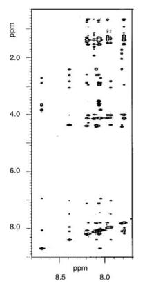
Figure 3.5 Partial NOESY spectrum of dynorphin A at 278 K in DMSO/water (80:20, v/v).
