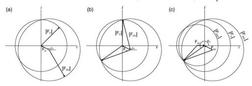
**Figure 2.16** Harker diagram showing the phase determination from isomorphous replacement. (a) Construct of a protein and protein soaked with heavy atom. Only the magnitudes of the structure factors are known ( $|\mathbf{F}_{P}|$  and  $|\mathbf{F}_{PH}|$ ), so they are drawn as circles with a radius corresponding to the magnitude. The vector with both magnitude and phase is drawn
