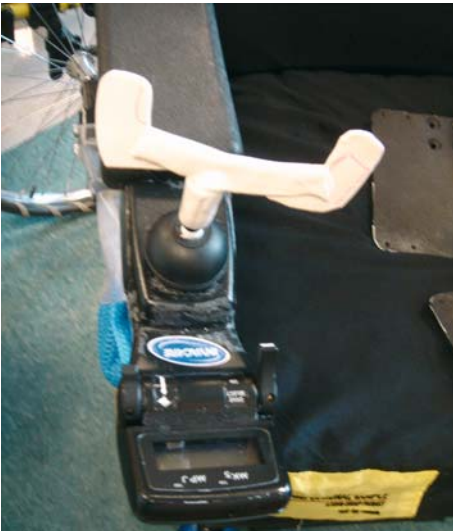
Fig. 12.5. Flap-like control paddle for SCI patient
