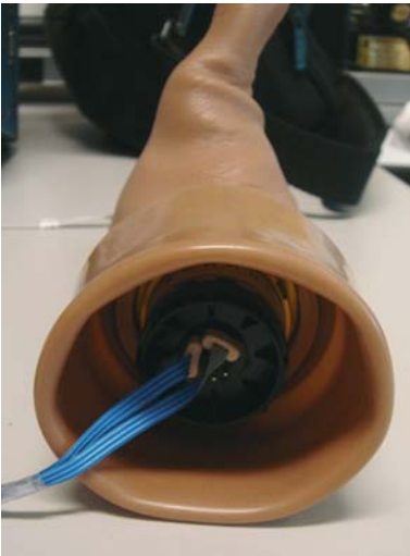
Fig. 6.5. The mechanical contraction of the residual stump muscles of the upper limb is transformed into EMG signals to operate the Otto-bock wrist unit, as shown here
