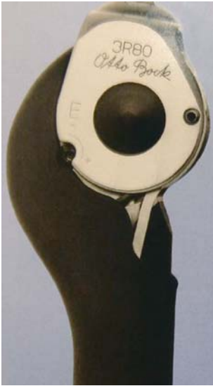
Fig. 10.8. Example of a prosthetic knee using the hydraulic system
