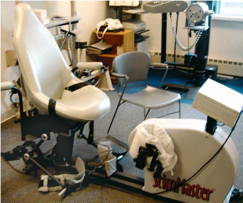
Fig. 12.7. Bicycle ergometer equipped with functional electrical stimulation (FES) capabilities
