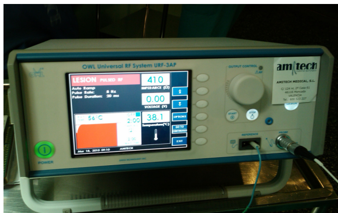
Fig. 1. RF generator: OWL universal RF System URP-3AP
