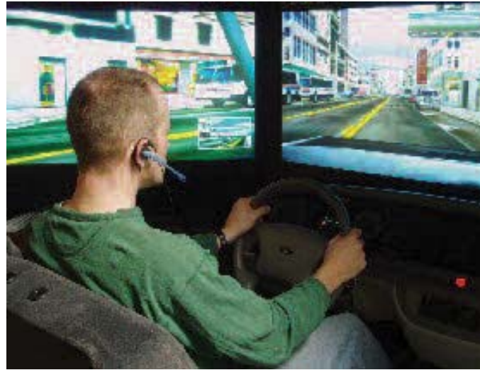
FIGURE 6.5 RESEARCH PARTICIPANT IN A COMPUTERIZED DRIVING SIMULATOR. The simulator provides a 180-degree city street interactive driving display in a realistic car interior. The “driver” is wearing a hands-free cell phone headset.
