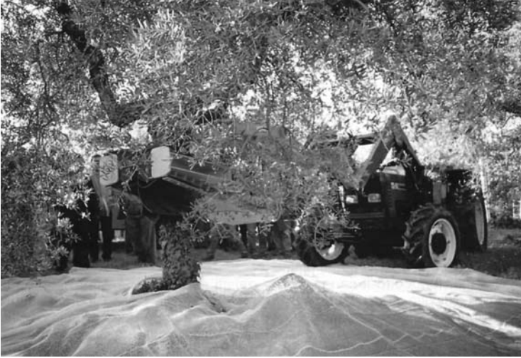
Fig. 22.3. Trunk shaker for olive harvesting. The fruits drop and are collected on a net or canvas placed under the tree canopy.
