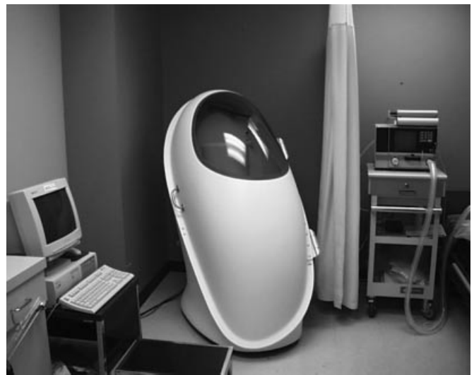
FIG. 58.1 An air-displacement plethysmograph located in the Department of Nutrition Sciences at the University of Alabama, Birmingham. Because the system measures pressure, it is important to house it in an area that does not experience rapid fluxes in air movement. This unit is housed in a room in which the room air circulation can be turned off during the measurement period, thereby decreasing measurement error.
