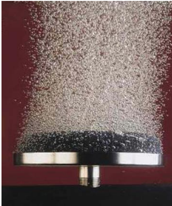
Plate 4.2 A fine bubble ozone diffuser in operation.
