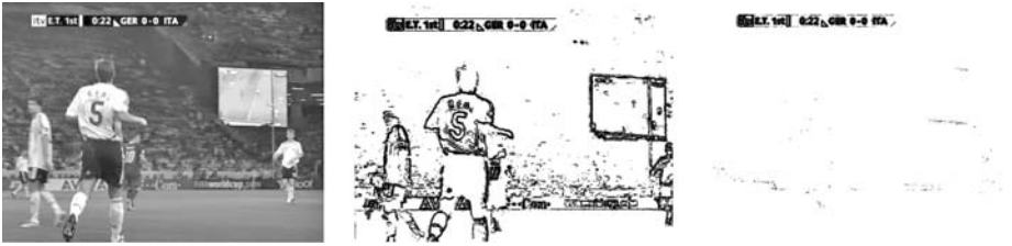
Figure 11.7 Detection of moving objects in soccer broadcasts. In the right-hand image all the moving objects have been removed.
