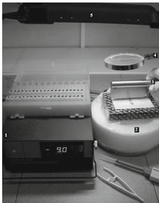
Fig. 3. An assembly for cutting SDS-PAGE gel slices; 1—power unit; 2—thermoelectric (a Peltier) cooler with glass plate ( 10 \times 7 \times 0.15 cm) on it; 3—a manual microtome R100 profile C; 4—magnifier (2 \times , d. 90–100 mm); 5—lamp for illumination of gel.
